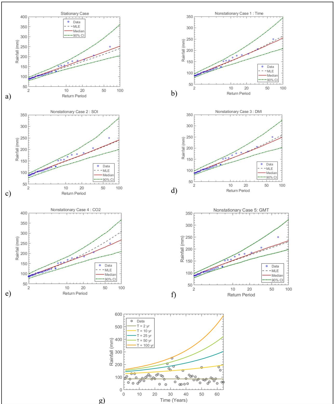
Figure 7.30 The GEV (a) stationary model, (b) non-stationary model considering time as a covariate, (c) non-stationary model considering SOI as a covariate, (d) non-stationary model considering DMI as a covariate, (e) non-stationary model considering CO<sub>2</sub> as a covariate, (f) non-stationary model considering GMT as a covariate and (g) effective return period as a function of time for Station 142: Eshowe – Brocklee Farm
