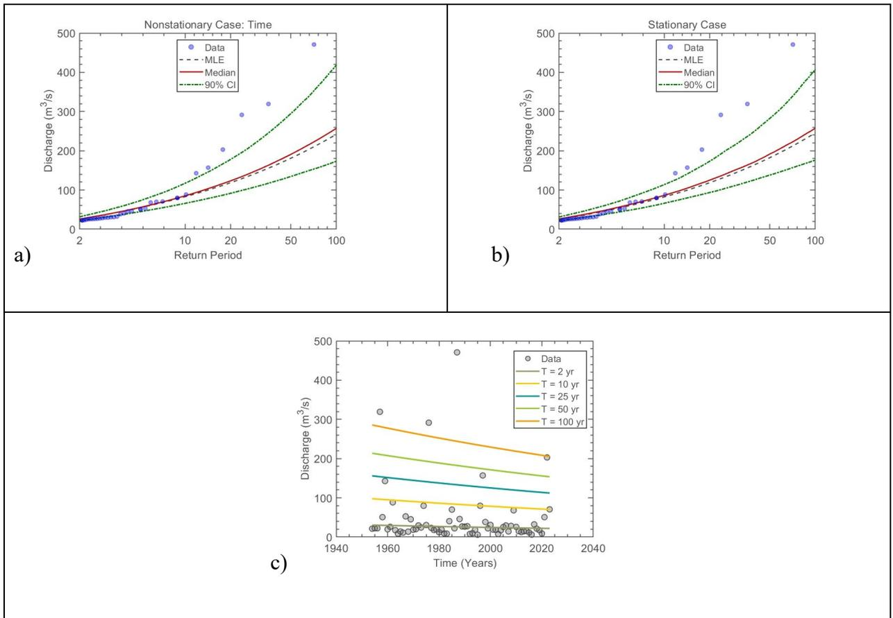
Figure 8.4 LP3 (a) stationary model, (b) non-stationary model considering time as a covariate, and (c) effective return period as a function of time for Station: U2H006
