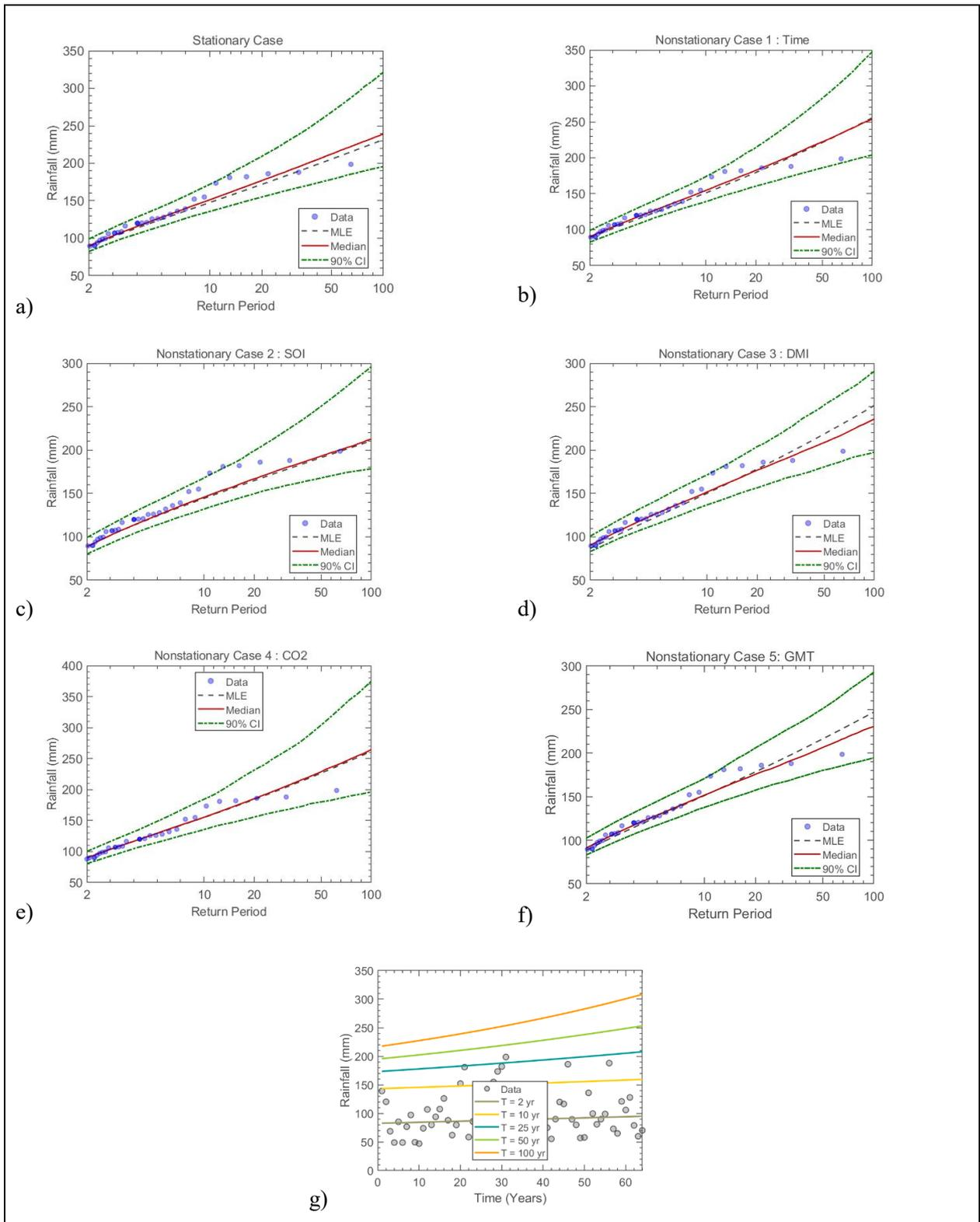
Figure 7.20 The GEV (a) stationary model, (b) non-stationary model considering time as a covariate, (c) non-stationary model considering SOI as a covariate, (d) non-stationary model considering DMI as a covariate, (e) non-stationary model considering CO<sub>2</sub> as a covariate, (f) non-stationary model considering GMT as a covariate and (g) effective return period as a function of time for Station 123: Maidstone – Sugar Mill (THS)
