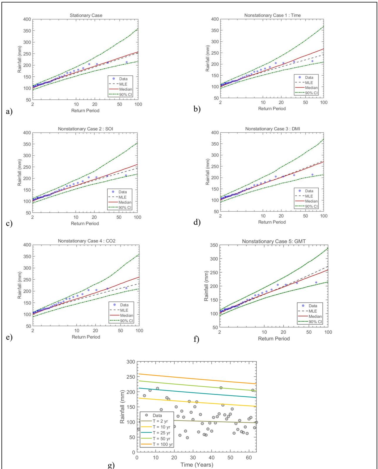
Figure 7.32 The GEV (a) stationary model, (b) non-stationary model considering time as a covariate, (c) non-stationary model considering SOI as a covariate, (d) non-stationary model considering DMI as a covariate, (e) non-stationary model considering CO<sub>2</sub> as a covariate, (f) non-stationary model considering GMT as a covariate and (g) effective return period as a function of time for Station 144: Felixton – Sugar Mill (THS)
