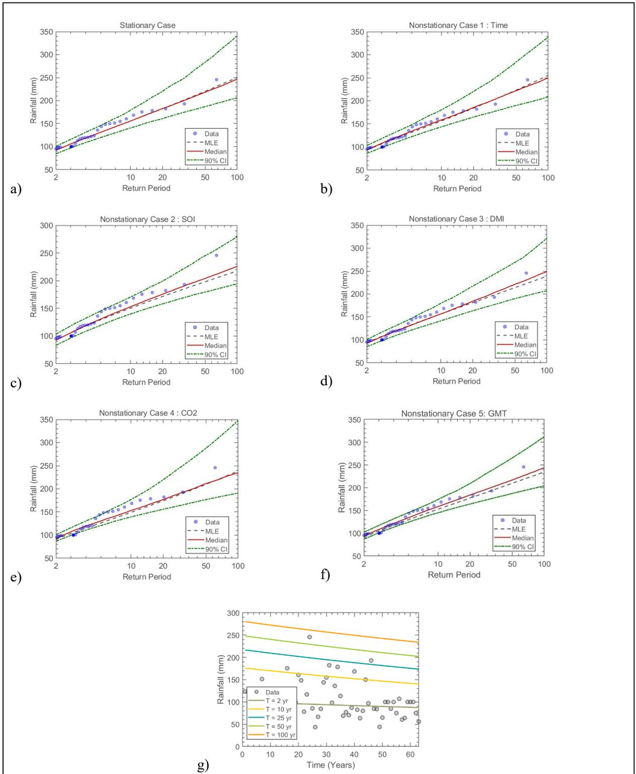
Figure 7.19 The GEV (a) stationary model, (b) non-stationary model considering time as a covariate, (c) non-stationary model considering SOI as a covariate, (d) non-stationary model considering DMI as a covariate, (e) non-stationary model considering CO<sub>2</sub> as a covariate, (f) non-stationary model considering GMT as a covariate and (g) effective return period as a function of time for Station 120: Inyaninga – THS
