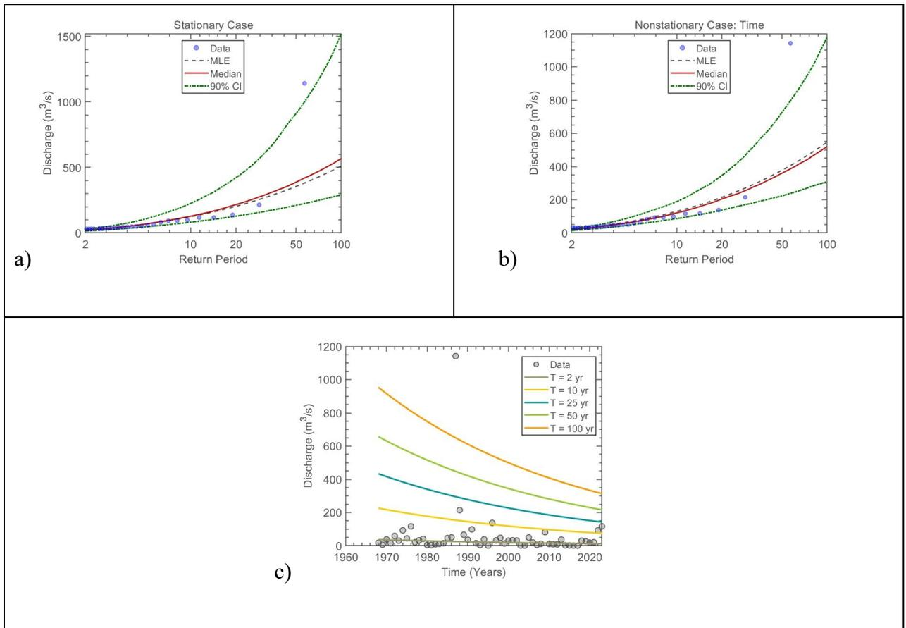
Figure 8.5 LP3 (a) stationary model, (b) non-stationary model considering time as a covariate, and (c) effective return period as a function of time for Station: U2H048
