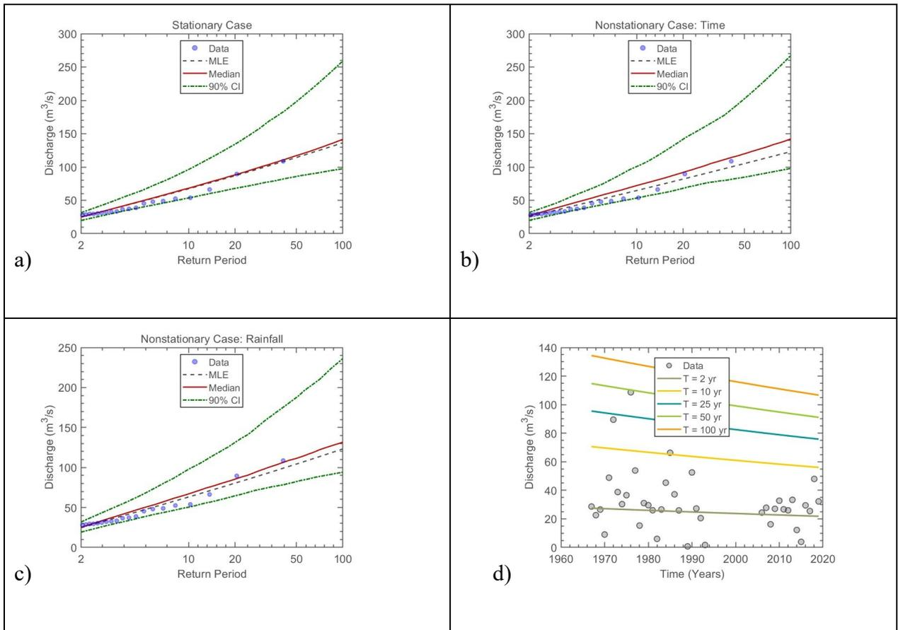
Figure 8.6 LP3 (a) stationary model, (b) non-stationary model considering time as a covariate, (c) non-stationary model considering rainfall as a covariate, and (d) effective return period as a function of time for Station:U3H001
