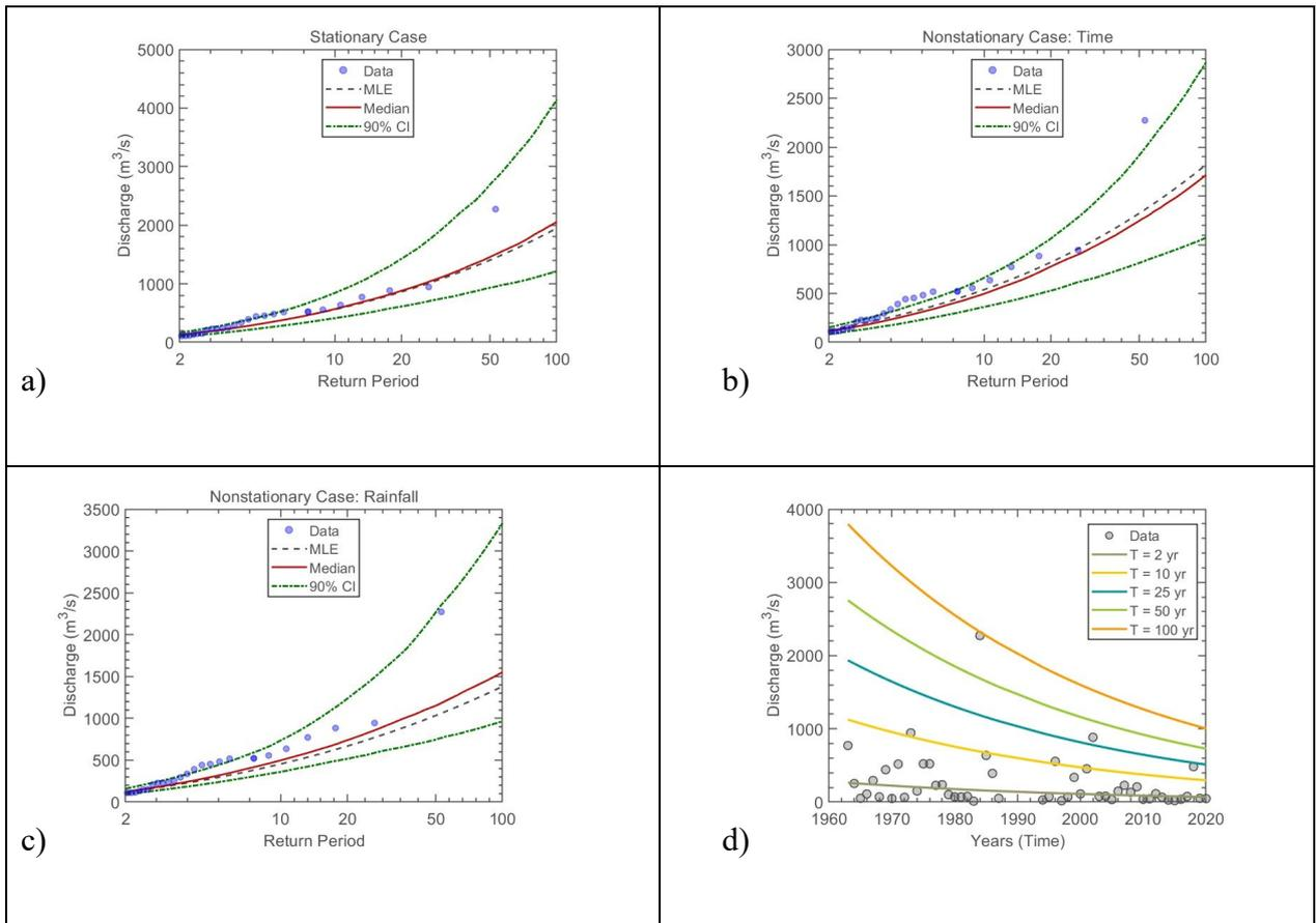
Figure 8.12 LP3 (a) stationary model, (b) non-stationary model considering time as a covariate, (c) non-stationary model considering rainfall as a covariate, and (d) effective return period as a function of time for Station:W1H009
