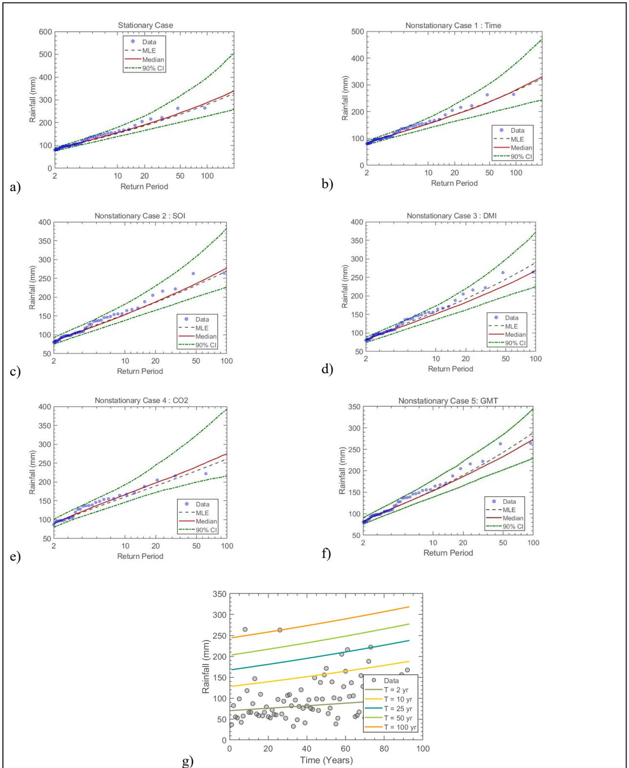
Figure 7.13 The GEV (a) stationary model, (b) non-stationary model considering time as a covariate, (c) non-stationary model considering SOI as a covariate, (d) non-stationary model considering DMI as a covariate, (e) non-stationary model considering CO<sub>2</sub> as a covariate, (f) non-stationary model considering GMT as a covariate and (g) effective return period as a function of time for Station 29: Mt Edgecombe – SASRI
