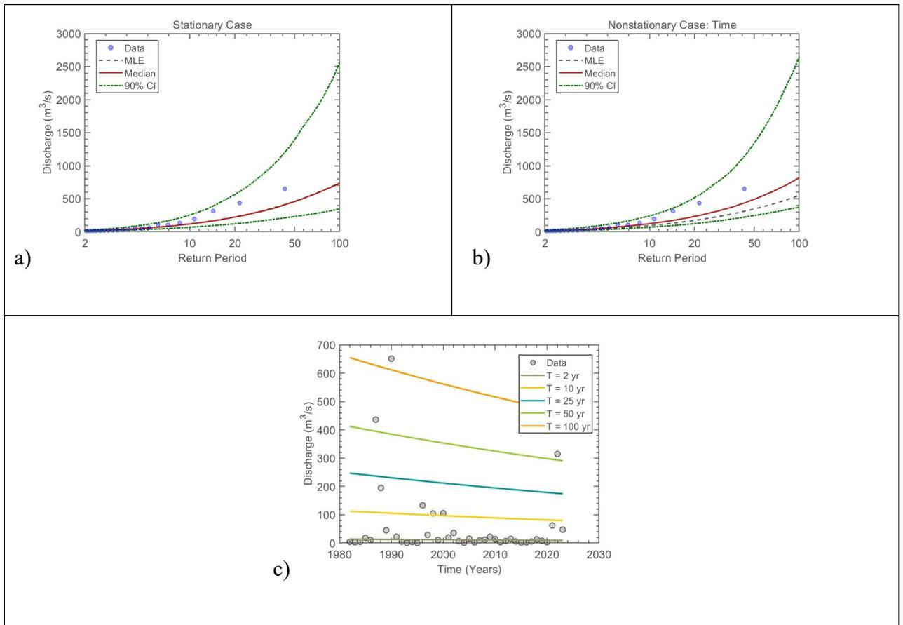
Figure 8.9 LP3 (a) stationary model, (b) non-stationary model considering time as a covariate, and (c) effective return period as a function of time for Station: U6H003
