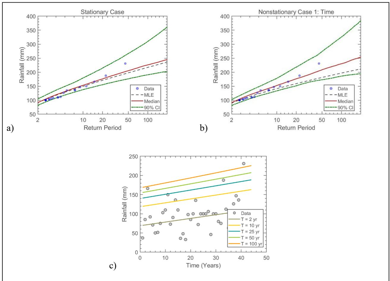
Figure 2.4 The GEV (a) stationary model, (b) non-stationary model considering time as a covariate, and (c) effective return period as a function of time for Station 38: Sezela - Illovo Sugar Estate
