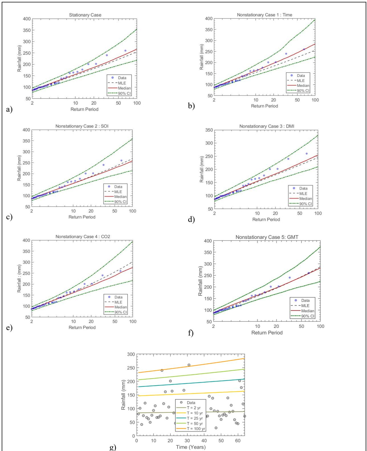
Figure 7.35 The GEV (a) stationary model, (b) non-stationary model considering time as a covariate, (c) non-stationary model considering SOI as a covariate, (d) non-stationary model considering DMI as a covariate, (e) non-stationary model considering CO<sub>2</sub> as a covariate, (f) non-stationary model considering GMT as a covariate and (g) effective return period as a function of time for Station 148: Mposa – Redcroft Farm
