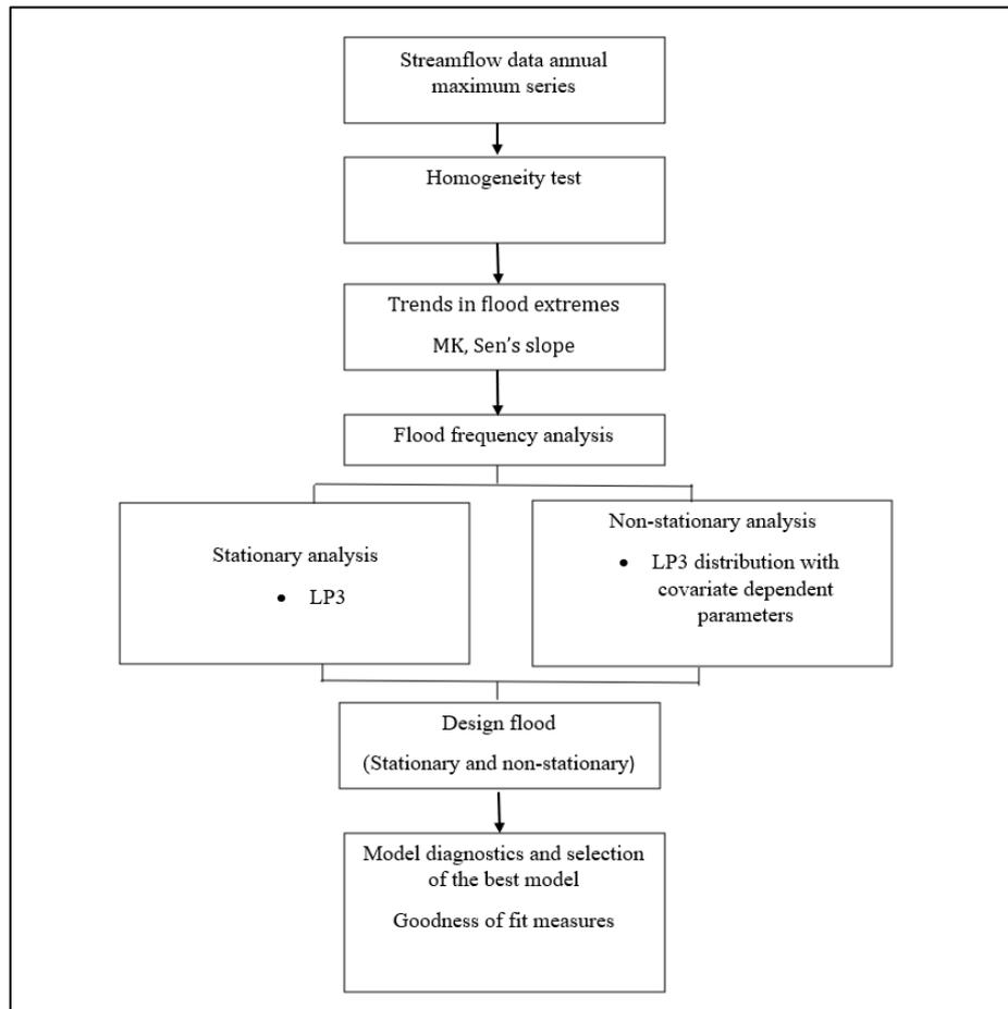
Figure 3.2 Stationary and non-stationary design flood estimation procedures
