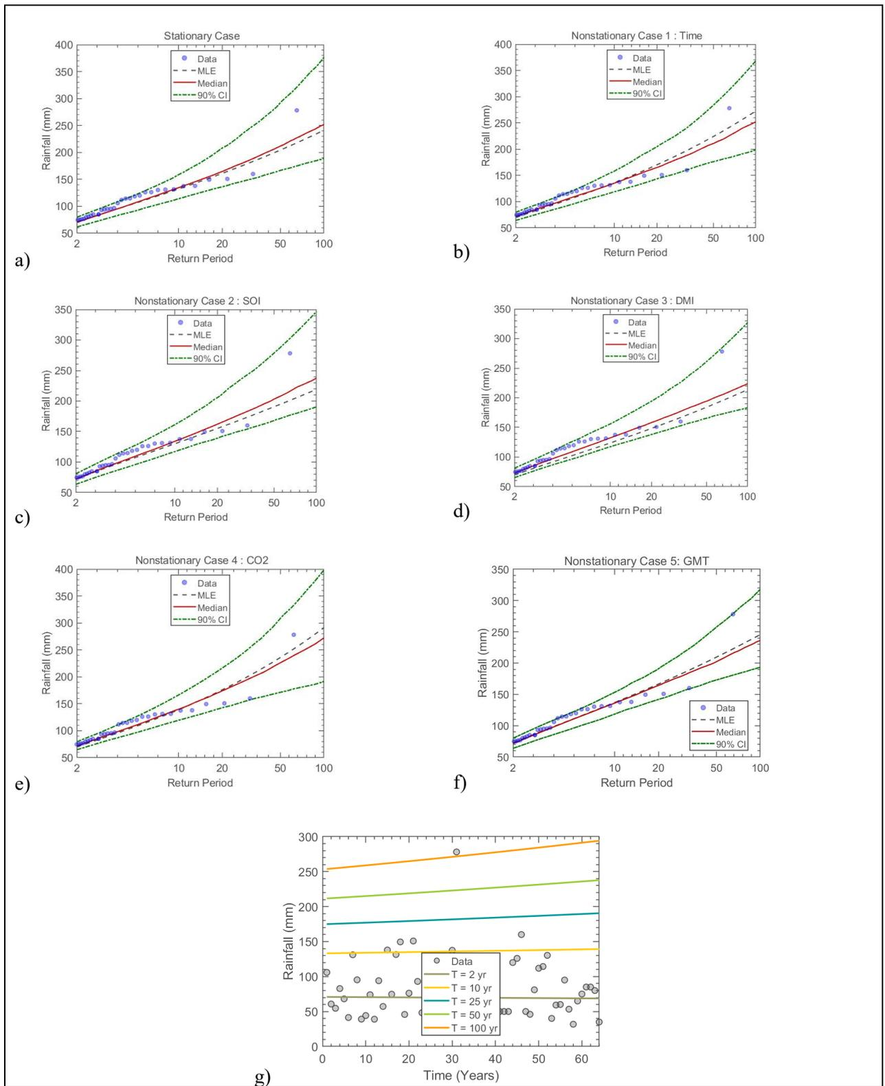
Figure 7.31 The GEV (a) stationary model, (b) non-stationary model considering time as a covariate, (c) non-stationary model considering SOI as a covariate, (d) non-stationary model considering DMI as a covariate, (e) non-stationary model considering CO<sub>2</sub> as a covariate, (f) non-stationary model considering GMT as a covariate and (g) effective return period as a function of time for Station 143: Nkwaleni – Zigagazi
