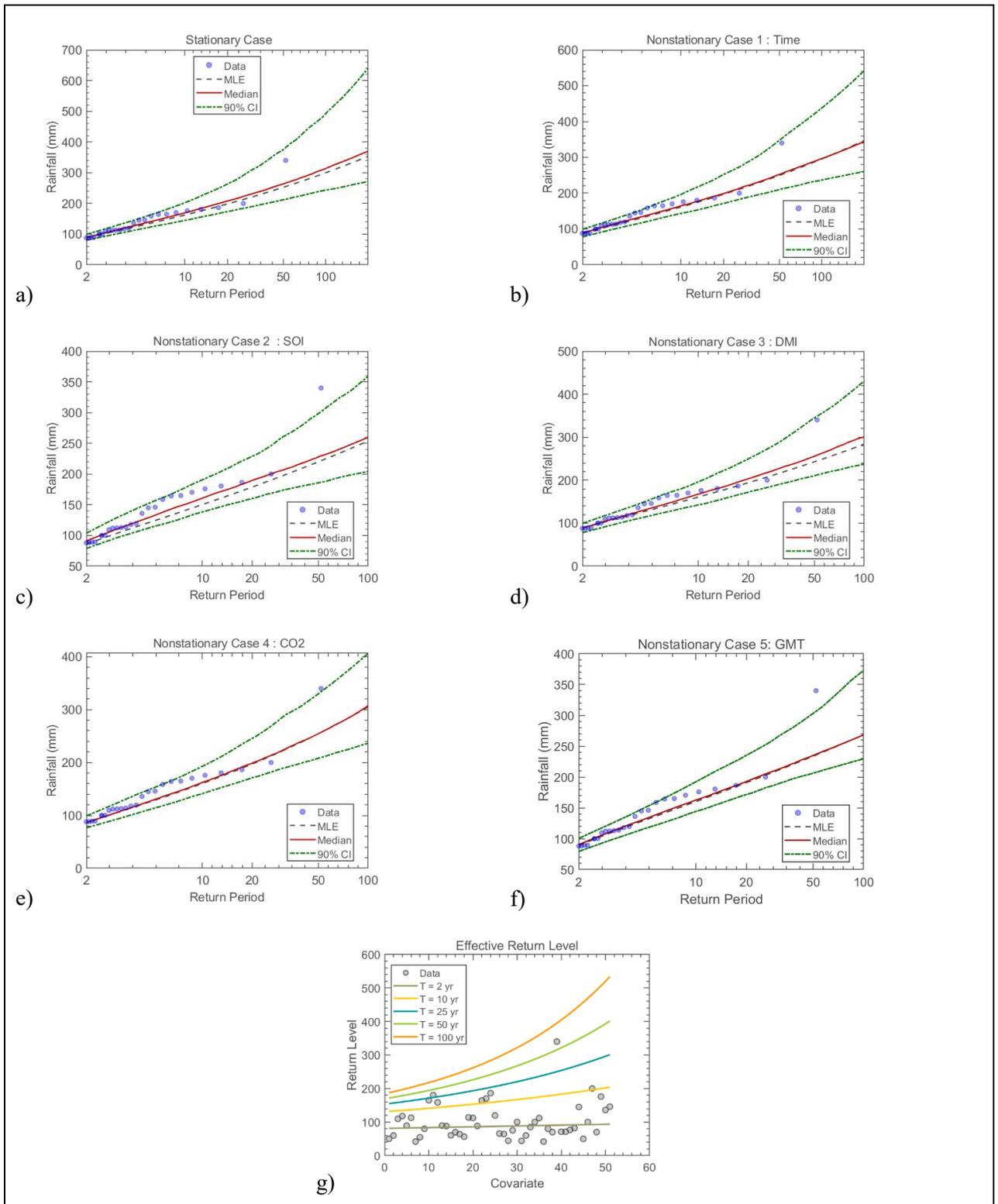
Figure 7.11 The GEV (a) stationary model, (b) non-stationary model considering time as a covariate, (c) non-stationary model considering SOI as a covariate, (d) non-stationary model considering DMI as a covariate, (e) non-stationary model considering CO<sub>2</sub> as a covariate, (f) non-stationary model considering GMT as a covariate and (g) effective return period as a function of time for Station 26: Illovo – Sugar Estate
