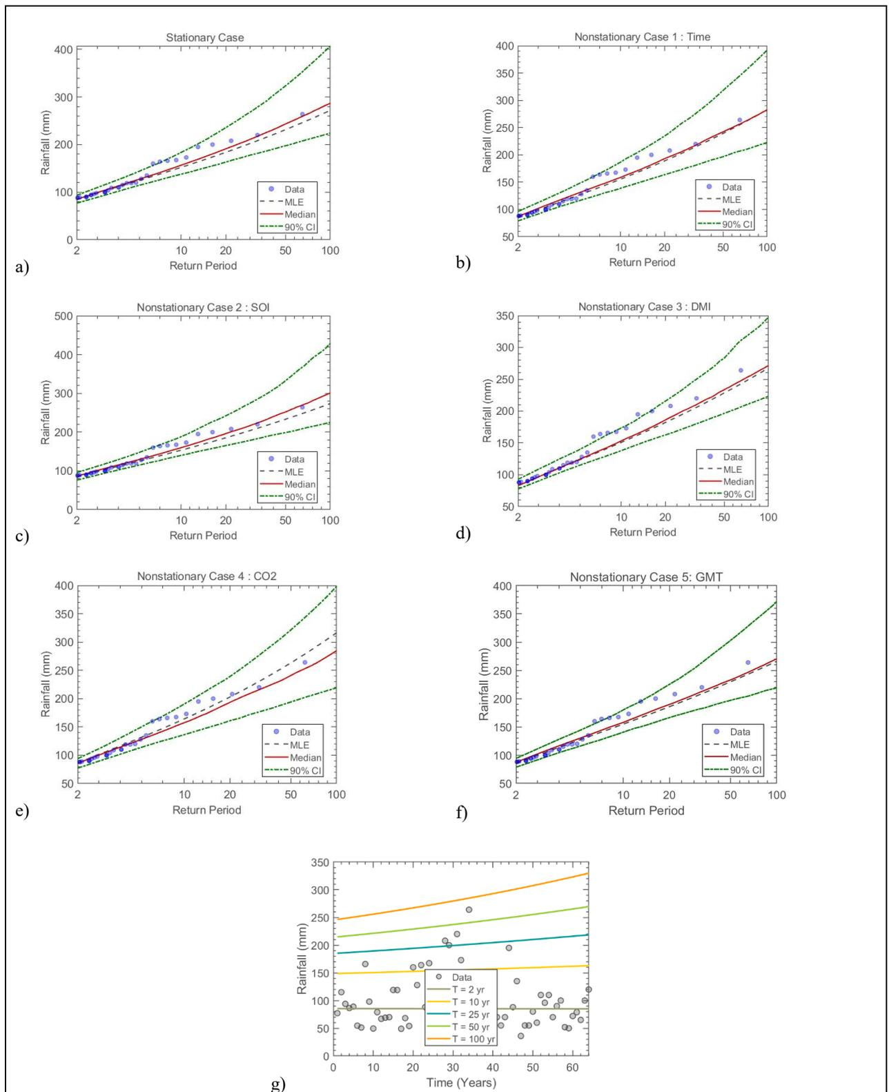
Figure 7.18 The GEV (a) stationary model, (b) non-stationary model considering time as a covariate, (c) non-stationary model considering SOI as a covariate, (d) non-stationary model considering DMI as a covariate, (e) non-stationary model considering CO<sub>2</sub> as a covariate, (f) non-stationary model considering GMT as a covariate and (g) effective return period as a function of time for Station 114: Inanda – Farm
