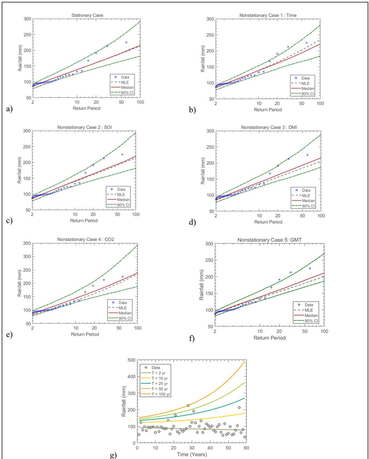
Figure 7.38 The GEV (a) stationary model, (b) non-stationary model considering time as a covariate, (c) non-stationary model considering SOI as a covariate, (d) non-stationary model considering DMI as a covariate, (e) non-stationary model considering CO<sub>2</sub> as a covariate, (f) non-stationary model considering GMT as a covariate and (g) effective return period as a function of time for Station 152: Mtubatuba – Nyalazi River
