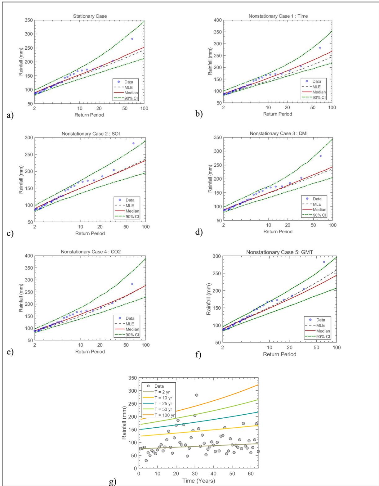
Figure 7.21 The GEV (a) stationary model, (b) non-stationary model considering time as a covariate, (c) non-stationary model considering SOI as a covariate, (d) non-stationary model considering DMI as a covariate, (e) non-stationary model considering CO<sub>2</sub> as a covariate, (f) non-stationary model considering GMT as a covariate and (g) effective return period as a function of time for Station 125: Sinembe – Spreyton Farm
