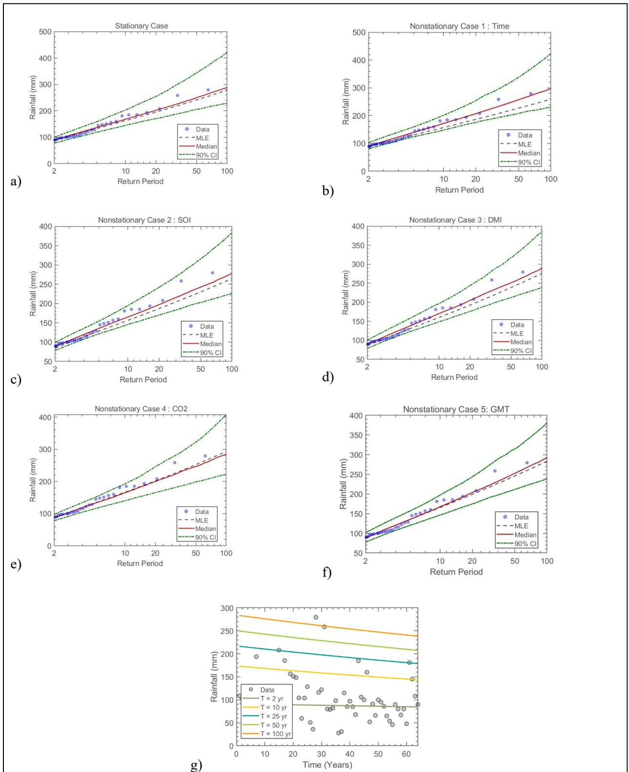
Figure 7.34 The GEV (a) stationary model, (b) non-stationary model considering time as a covariate, (c) non-stationary model considering SOI as a covariate, (d) non-stationary model considering DMI as a covariate, (e) non-stationary model considering CO<sub>2</sub> as a covariate, (f) non-stationary model considering GMT as a covariate and (g) effective return period as a function of time for Station 147: Ukulu Properties – Crystal Holdings
