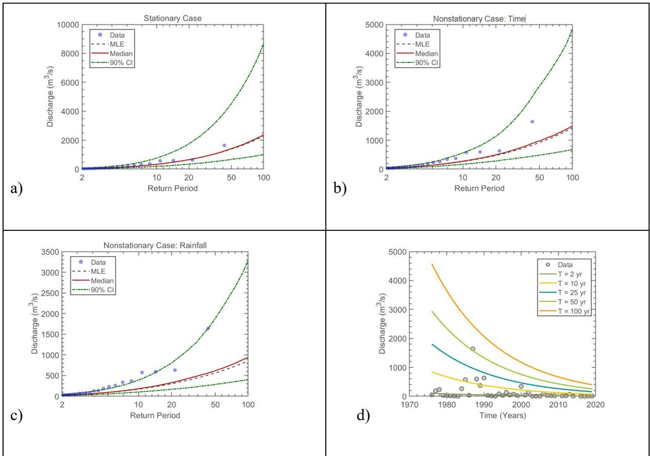
Figure 8.7 LP3 (a) stationary model, (b) non-stationary model considering time as a covariate, (c) non-stationary model considering rainfall as a covariate, and (d) effective return period as a function of time for Station:U3H005
