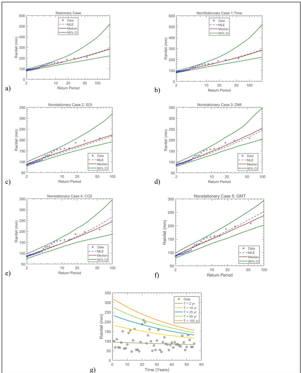
Figure 7.8 The GEV (a) stationary model, (b) non-stationary model considering time as a covariate, (c) non-stationary model considering SOI as a covariate, (d) non-stationary model considering DMI as a covariate, (e) non-stationary model considering CO<sub>2</sub> as a covariate, (f) non-stationary model considering GMT as a covariate and (g) effective return period as a function of time for Station 20: Tongaat – Klipfontein (THS)
