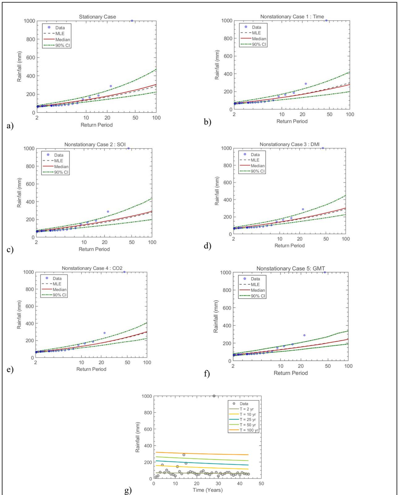
Figure 7.27 The GEV (a) stationary model, (b) non-stationary model considering time as a covariate, (c) non-stationary model considering SOI as a covariate, (d) non-stationary model considering DMI as a covariate, (e) non-stationary model considering CO<sub>2</sub> as a covariate, (f) non-stationary model considering GMT as a covariate and (g) effective return period as a function of time for Station 136: Glenside – Misty Krantz Estate
