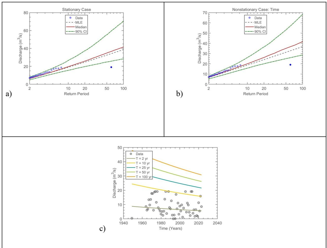
Figure 8.8 LP3 (a) stationary model, (b) non-stationary model considering time as a covariate, and (c) effective return period as a function of time for Station: U4H002
