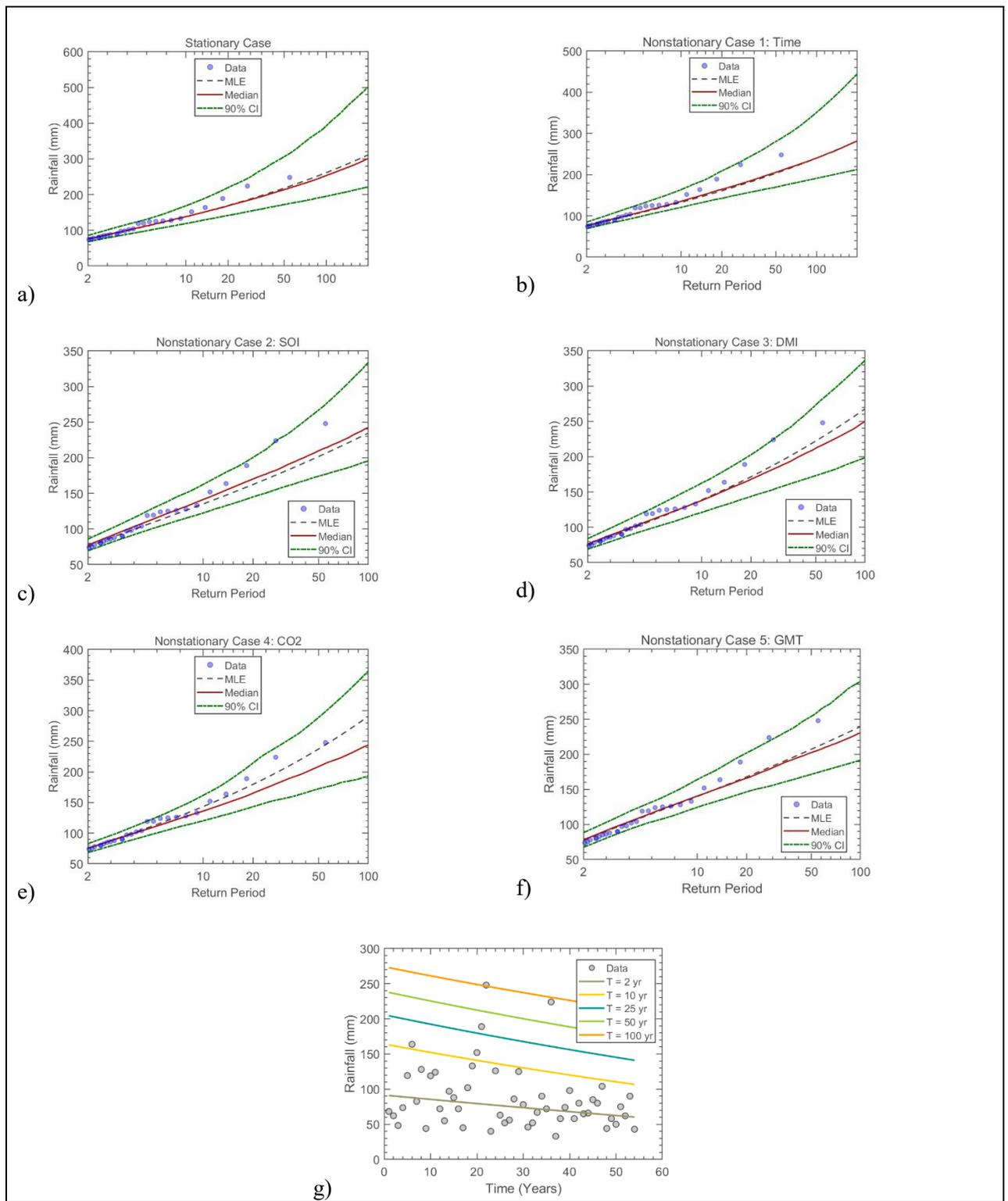
Figure 7.7 The GEV (a) stationary model, (b) non-stationary model considering time as a covariate, (c) non-stationary model considering SOI as a covariate, (d) non-stationary model considering DMI as a covariate, (e) non-stationary model considering CO<sub>2</sub> as a covariate, (f) non-stationary model considering GMT as a covariate and (g) effective return period as a function of time for Station 18: Glendale – Tenrith Farm
