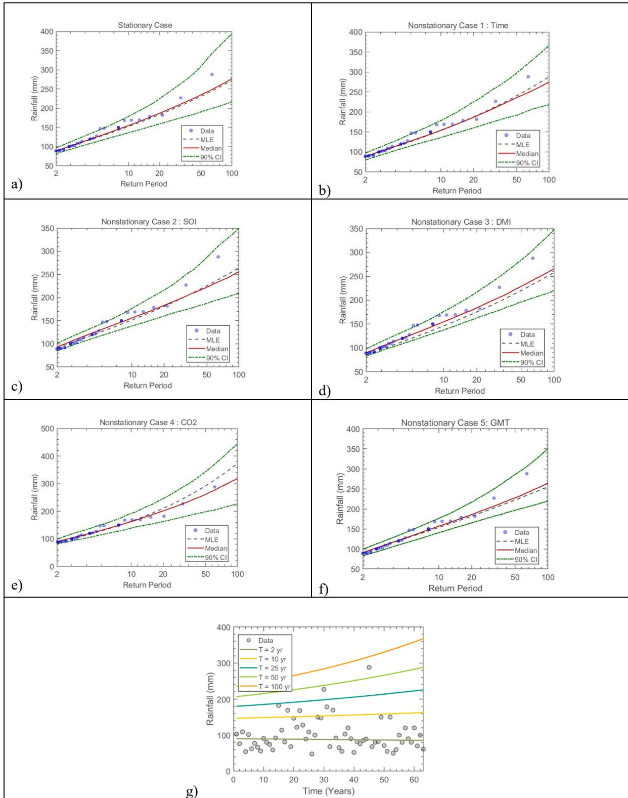
Figure 7.24 The GEV (a) stationary model, (b) non-stationary model considering time as a covariate, (c) non-stationary model considering SOI as a covariate, (d) non-stationary model considering DMI as a covariate, (e) non-stationary model considering CO<sub>2</sub> as a covariate, (f) non-stationary model considering GMT as a covariate and (g) effective return period as a function of time for Station 130: Doornkop – Langespruit Farm
