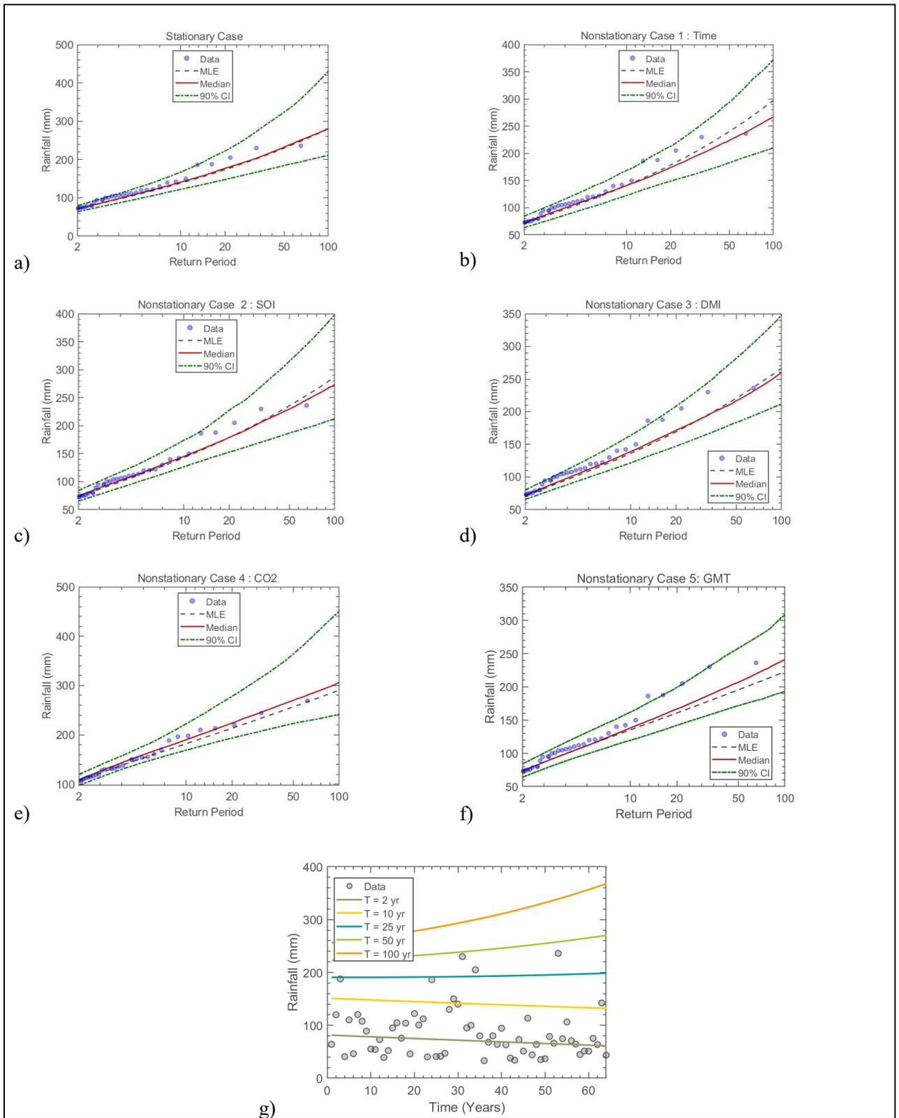
Figure 7.17 The GEV (a) stationary model, (b) non-stationary model considering time as a covariate, (c) non-stationary model considering SOI as a covariate, (d) non-stationary model considering DMI as a covariate, (e) non-stationary model considering CO<sub>2</sub> as a covariate, (f) non-stationary model considering GMT as a covariate and (g) effective return period as a function of time for Station 111: Powerscourt – Roseleigh Estate
