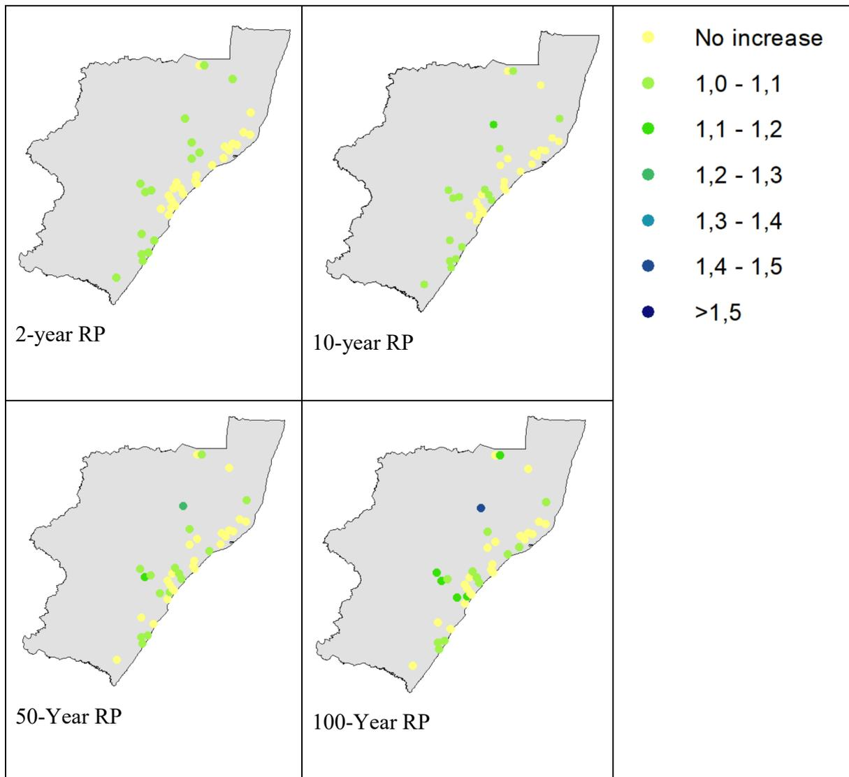
Figure 2.7 Projected changes from the present to the near future in design rainfalls for 1-day design rainfalls for the 2-, 10-, 50-, and 100-year return periods, derived from outputs from multiple GCMs
