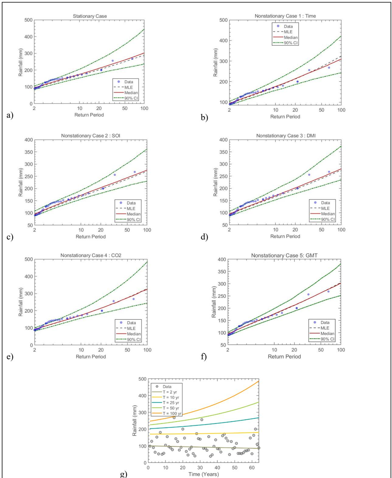
Figure 7.33 The GEV (a) stationary model, (b) non-stationary model considering time as a covariate, (c) non-stationary model considering SOI as a covariate, (d) non-stationary model considering DMI as a covariate, (e) non-stationary model considering CO<sub>2</sub> as a covariate, (f) non-stationary model considering GMT as a covariate and (g) effective return period as a function of time for Station 146: Kulu Halt – Honey Farm
