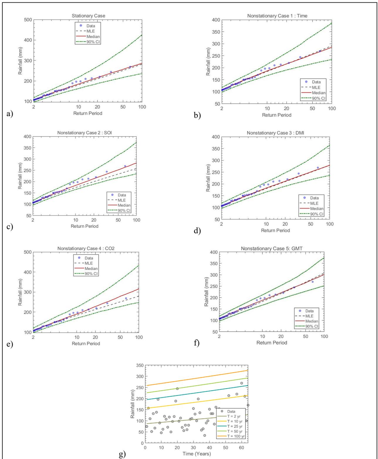
Figure 7.16 The GEV (a) stationary model, (b) non-stationary model considering time as a covariate, (c) non-stationary model considering SOI as a covariate, (d) non-stationary model considering DMI as a covariate, (e) non-stationary model considering CO<sub>2</sub> as a covariate, (f) non-stationary model considering GMT as a covariate and (g) effective return period as a function of time for Station 110: Renishaw – Crooks Bros Estate
