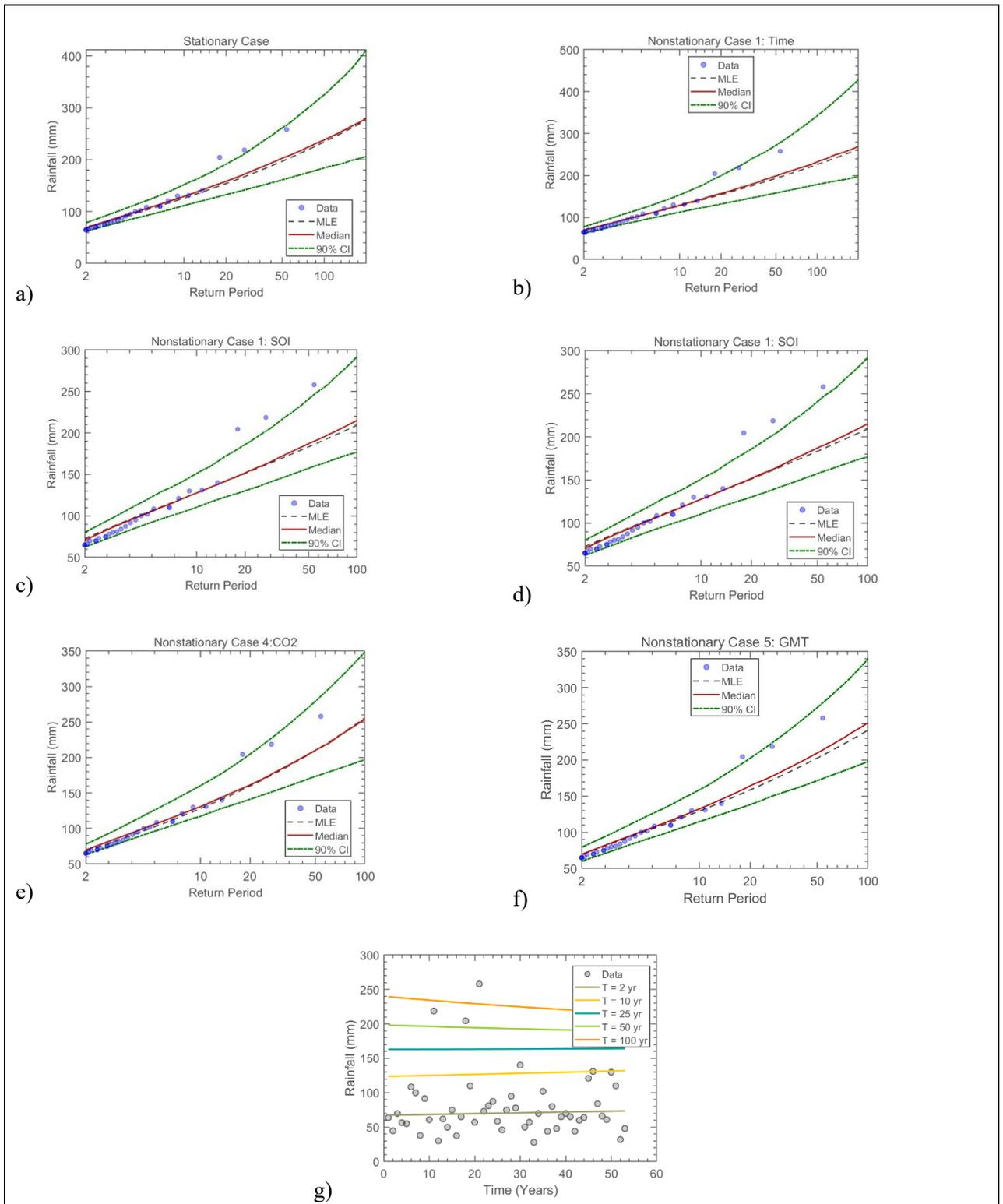
Figure 7.6 The GEV (a) stationary model, (b) non-stationary model considering time as a covariate, (c) non-stationary model considering SOI as a covariate, (d) non-stationary model considering DMI as a covariate, (e) non-stationary model considering CO<sub>2</sub> as a covariate, (f) non-stationary model considering GMT as a covariate and (g) effective return period as a function of time for Station 12: Melmoth – CA Leith & Sons
