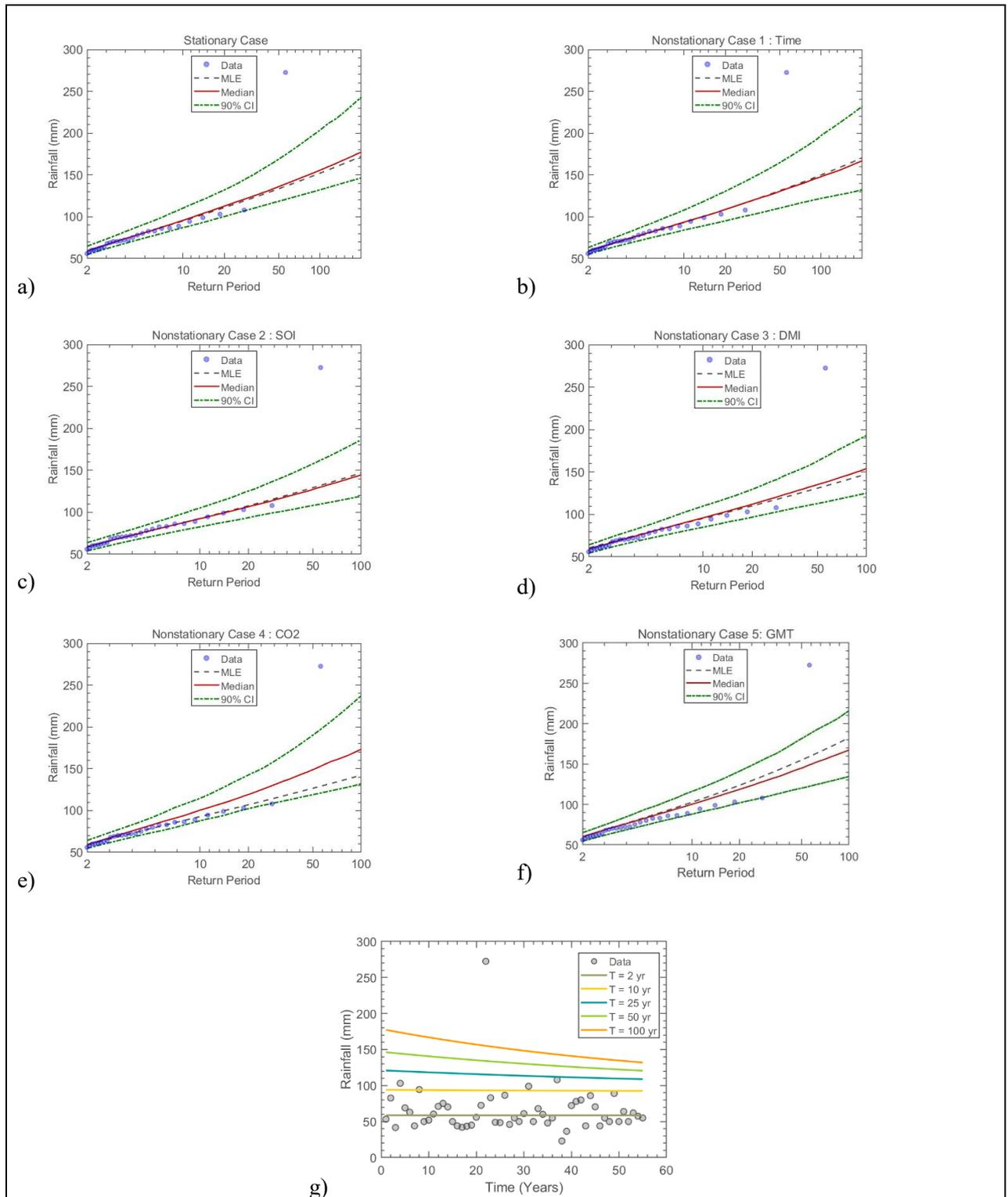
Figure 7.9 The GEV (a) stationary model, (b) non-stationary model considering time as a covariate, (c) non-stationary model considering SOI as a covariate, (d) non-stationary model considering DMI as a covariate, (e) non-stationary model considering CO<sub>2</sub> as a covariate, (f) non-stationary model considering GMT as a covariate and (g) effective return period as a function of time for Station 22: Seven Oaks – Saw Mill
