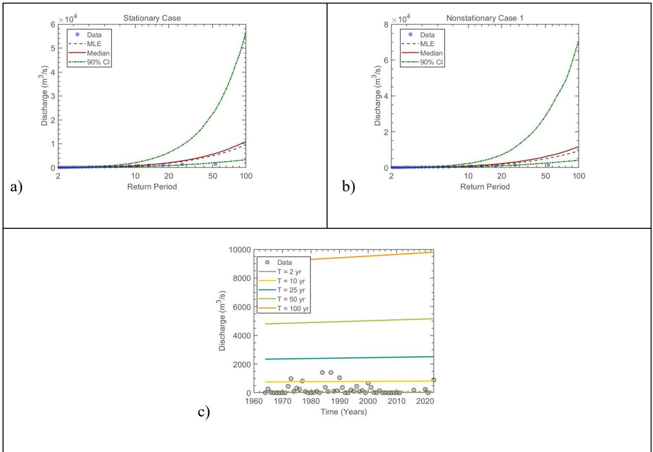
Figure 8.14 LP3 (a) stationary model, (b) non-stationary model considering time as a covariate, and (c) effective return period as a function of time for Station: W3H022
