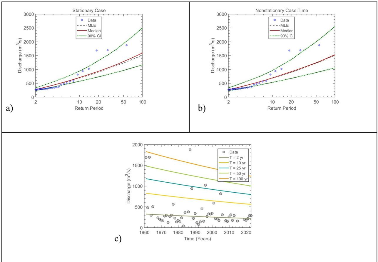
Figure 8.13 LP3 (a) stationary model, (b) non-stationary model considering time as a covariate, and (c) effective return period as a function of time for Station: W2H005
