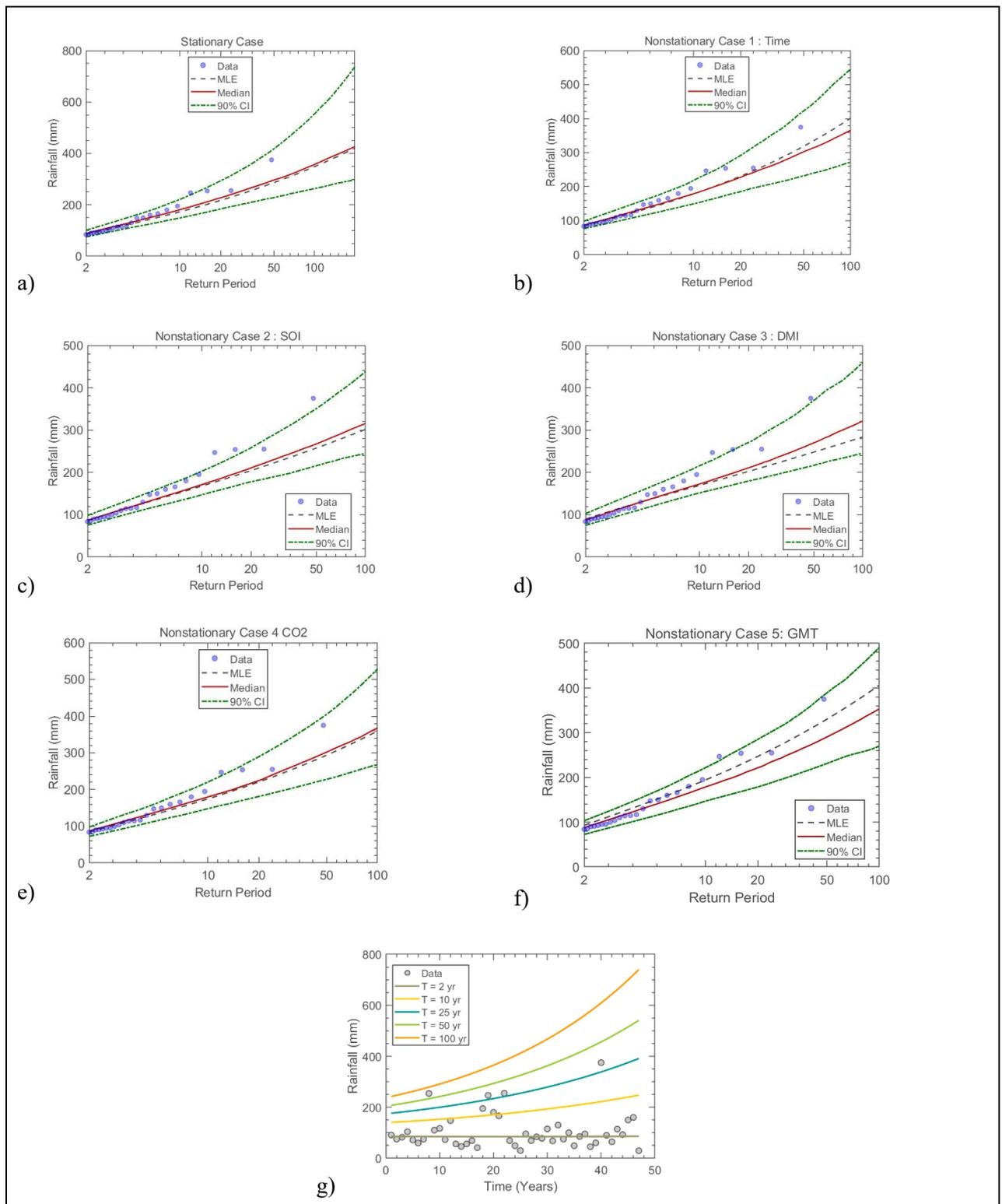
Figure 7.12 The GEV (a) stationary model, (b) non-stationary model considering time as a covariate, (c) non-stationary model considering SOI as a covariate, (d) non-stationary model considering DMI as a covariate, (e) non-stationary model considering CO<sub>2</sub> as a covariate, (f) non-stationary model considering GMT as a covariate and (g) effective return period as a function of time for Station 27: Vulamehlo – Esperanza
