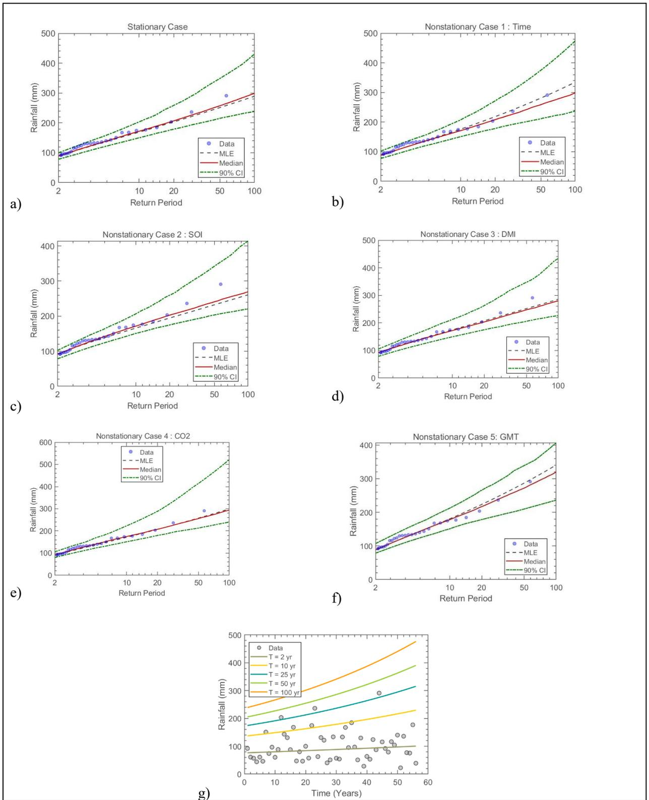
Figure 7.15 The GEV (a) stationary model, (b) non-stationary model considering time as a covariate, (c) non-stationary model considering SOI as a covariate, (d) non-stationary model considering DMI as a covariate, (e) non-stationary model considering CO<sub>2</sub> as a covariate, (f) non-stationary model considering GMT as a covariate and (g) effective return period as a function of time for Station 105: Oribi Flats – Minnehaha Farm
