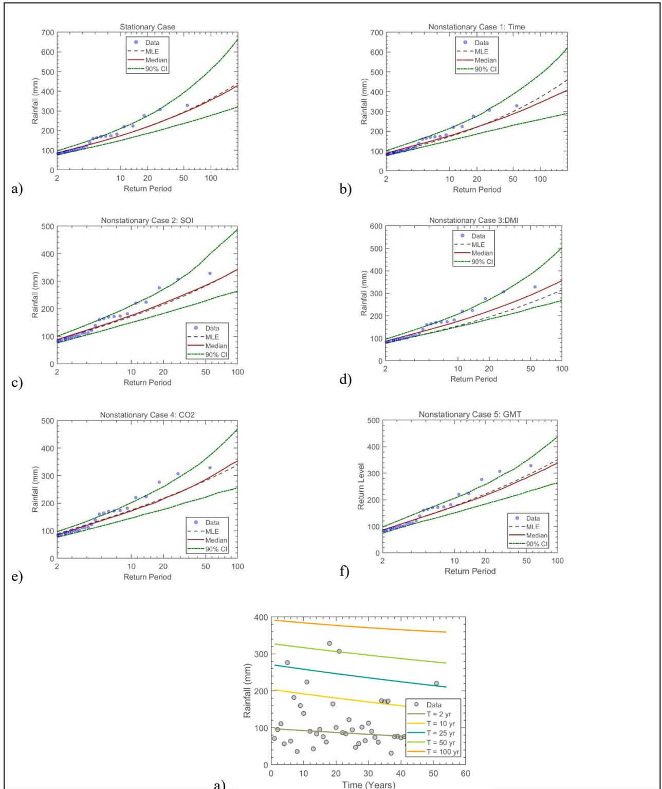
Figure 7.4 The GEV (a) stationary model, (b) non-stationary model considering time as a covariate, (c) non-stationary model considering SOI as a covariate, (d) non-stationary model considering DMI as a covariate, (e) non-stationary model considering CO<sub>2</sub> as a covariate, (f) non-stationary model considering GMT as a covariate and (g) effective return period as a function of time for Station 9: Mtubatuba – Riverview Sugar Mill
