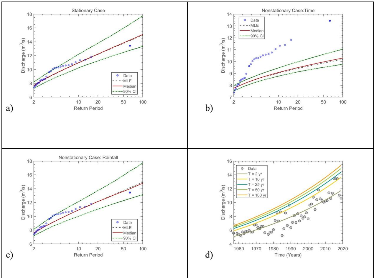
Figure 8.15 LP3 (a) stationary model, (b) non-stationary model considering time as a covariate, (c) non-stationary model considering rainfall as a covariate, and (d) effective return period as a function of time for Station:W4H012
