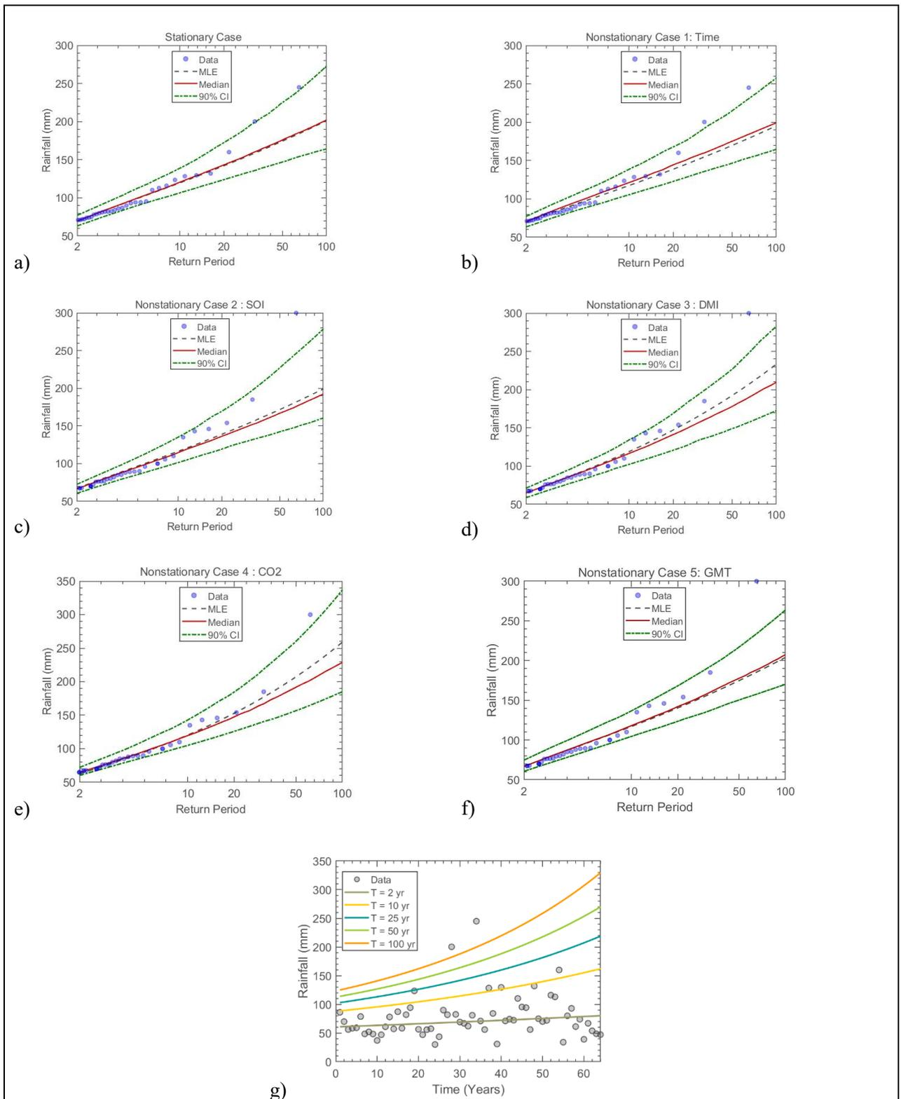
Figure 7.40 The GEV (a) stationary model, (b) non-stationary model considering time as a covariate, (c) non-stationary model considering SOI as a covariate, (d) non-stationary model considering DMI as a covariate, (e) non-stationary model considering CO<sub>2</sub> as a covariate, (f) non-stationary model considering GMT as a covariate and (g) effective return period as a function of time for Station 155: Pongola – Impala Irrigation Board
