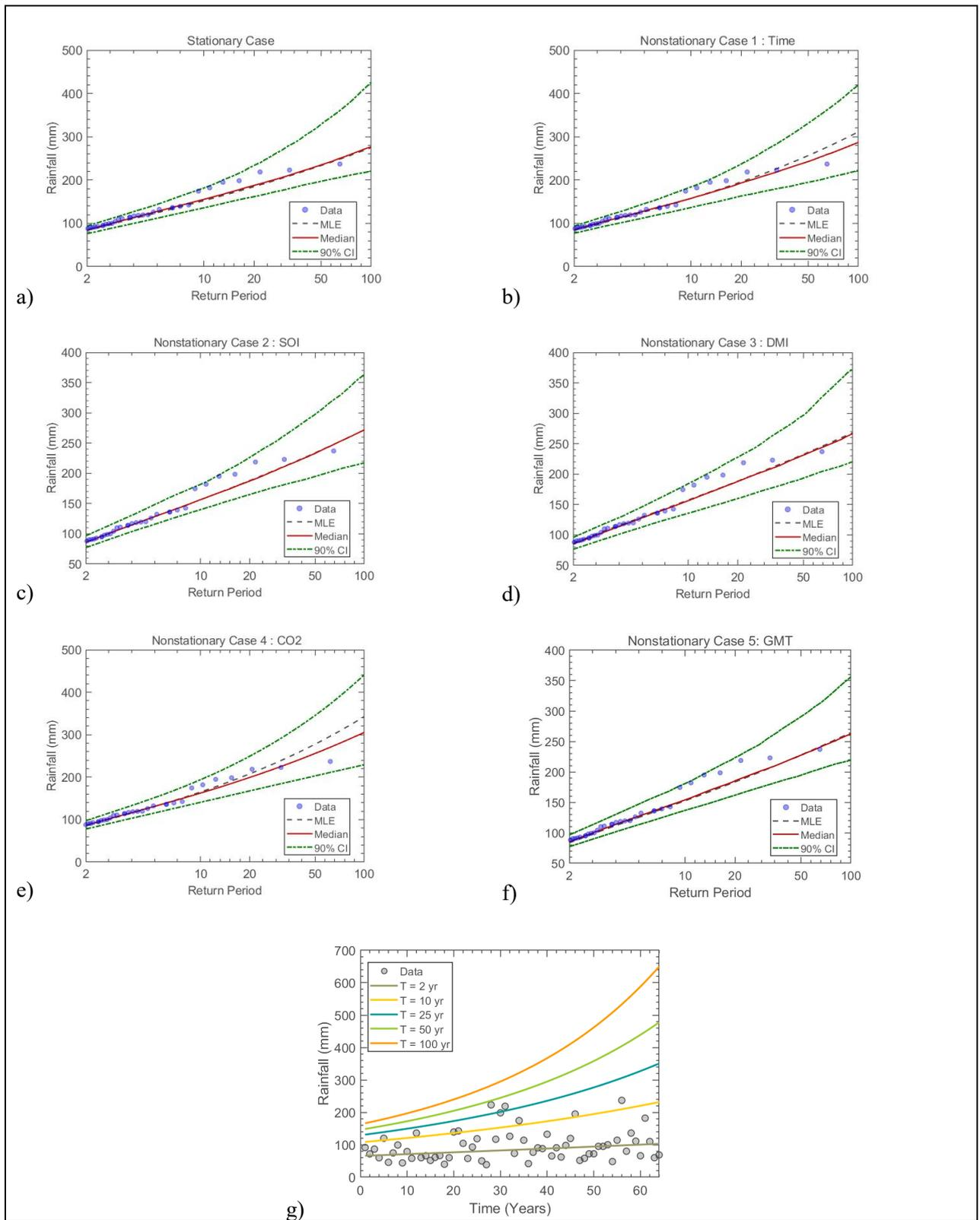
Figure 7.29 The GEV (a) stationary model, (b) non-stationary model considering time as a covariate, (c) non-stationary model considering SOI as a covariate, (d) non-stationary model considering DMI as a covariate, (e) non-stationary model considering CO<sub>2</sub> as a covariate, (f) non-stationary model considering GMT as a covariate and (g) effective return period as a function of time for Station 139: Inyoni – Myrln Estate
