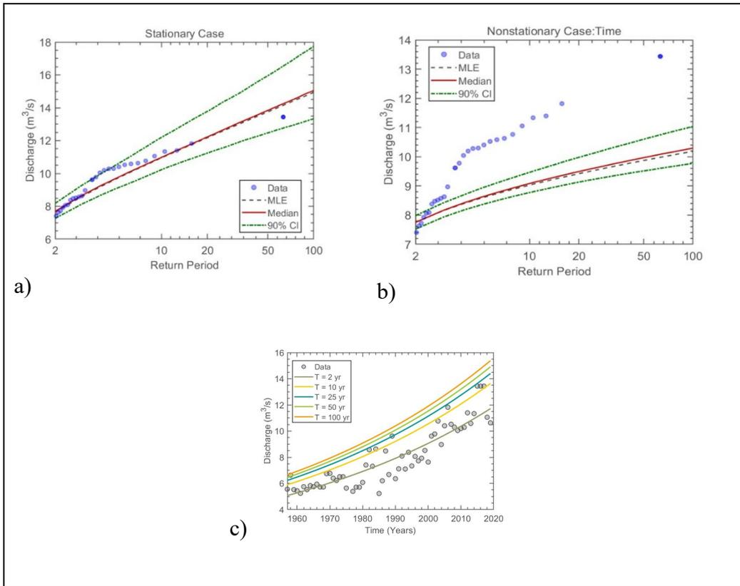
Figure 3.3 The LP3 (a) stationary model, (b) non-stationary model considering time as a covariate, and (c) effective return period as a function of time for Station W4H012
