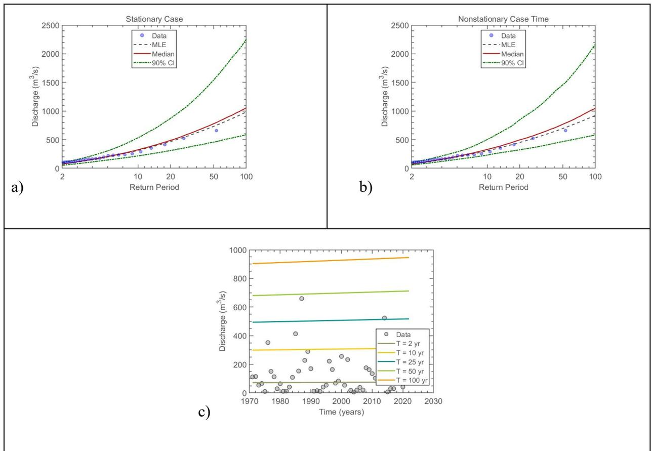
Figure 8.2 The LP3 (a) stationary model, (b) non-stationary model considering time as a covariate, and (c) effective return period as a function of time for Station: T5H012
