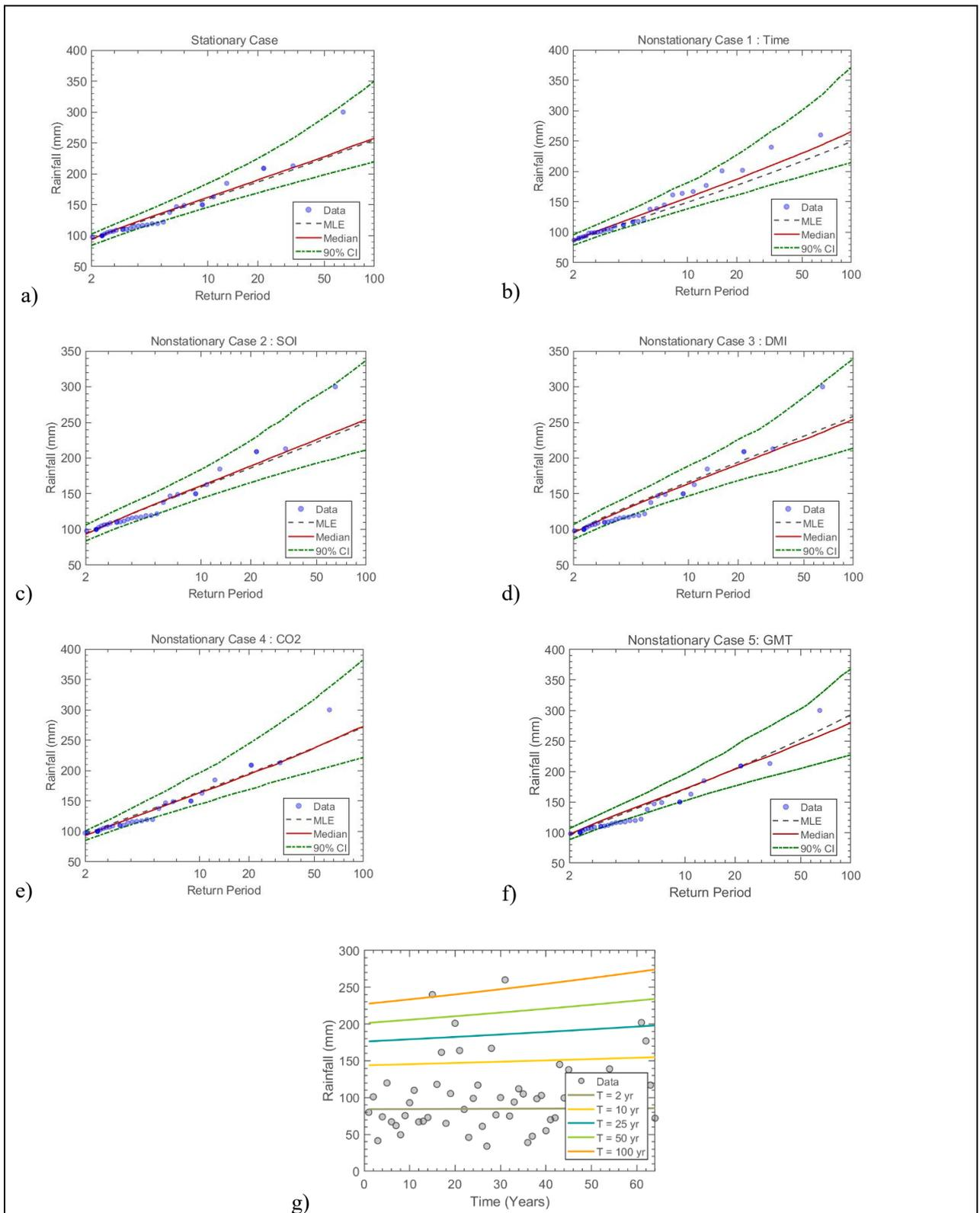
Figure 7.36 The GEV (a) stationary model, (b) non-stationary model considering time as a covariate, (c) non-stationary model considering SOI as a covariate, (d) non-stationary model considering DMI as a covariate, (e) non-stationary model considering CO<sub>2</sub> as a covariate, (f) non-stationary model considering GMT as a covariate and (g) effective return period as a function of time for Station 149: Kwambonambi – Mondi Forestry
