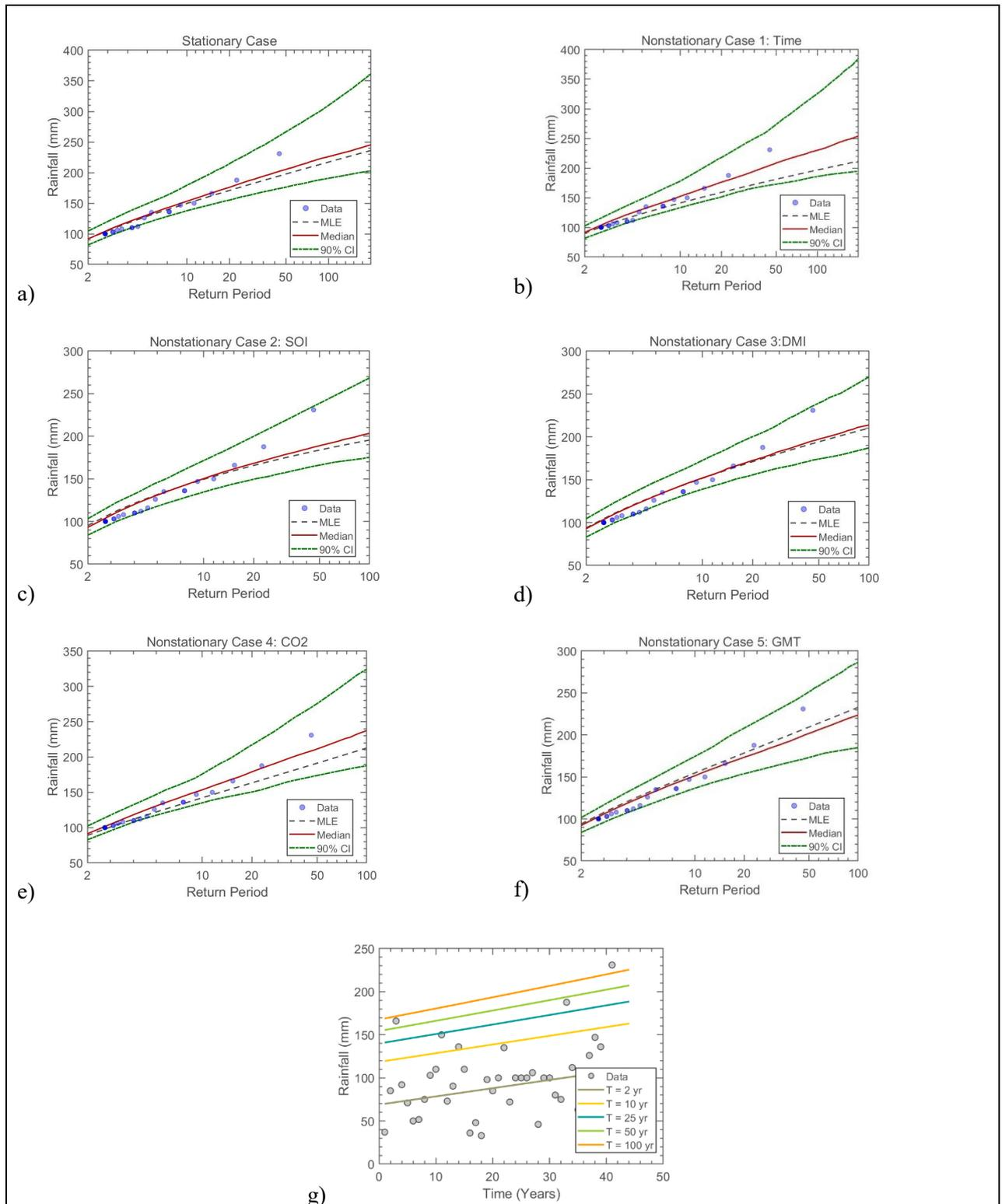
Figure 7.14 The GEV (a) stationary model, (b) non-stationary model considering time as a covariate, (c) non-stationary model considering SOI as a covariate, (d) non-stationary model considering DMI as a covariate, (e) non-stationary model considering CO<sub>2</sub> as a covariate, (f) non-stationary model considering GMT as a covariate and (g) effective return period as a function of time for Station 38: Sezela – Illovo Sugar Estate
