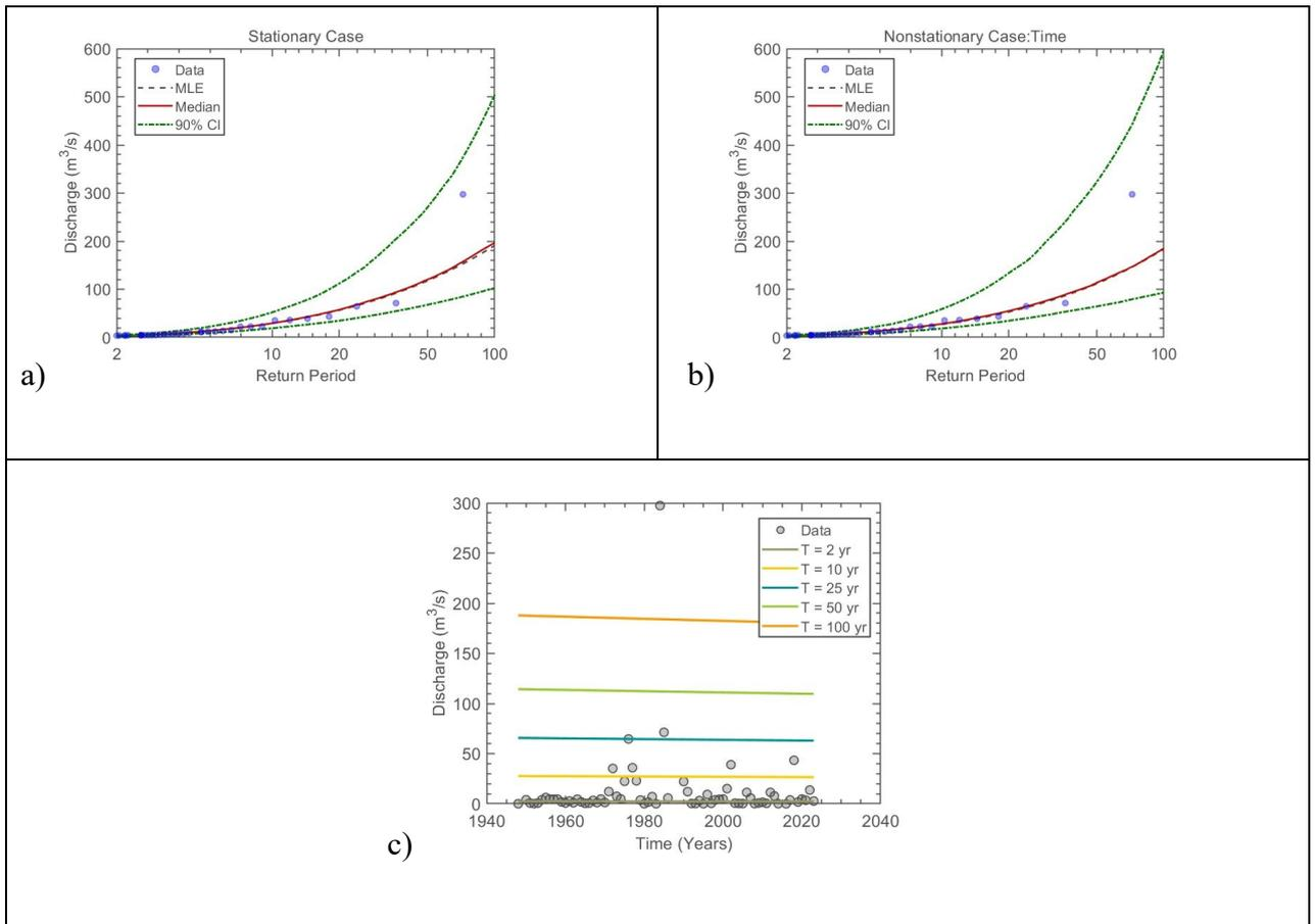
Figure 8.11 LP3 (a) stationary model, (b) non-stationary model considering time as a covariate, and (c) effective return period as a function of time for Station: W1H004
