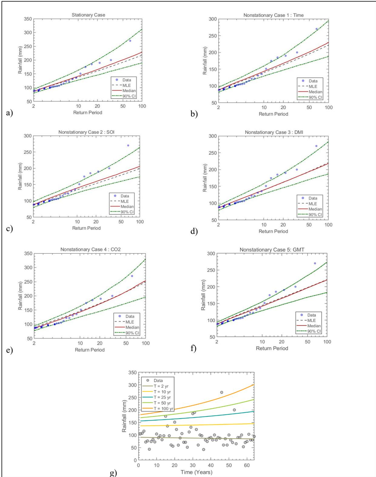
Figure 7.23 The GEV (a) stationary model, (b) non-stationary model considering time as a covariate, (c) non-stationary model considering SOI as a covariate, (d) non-stationary model considering DMI as a covariate, (e) non-stationary model considering CO<sub>2</sub> as a covariate, (f) non-stationary model considering GMT as a covariate and (g) effective return period as a function of time for Station 129: Kearsney – Ocean Lodge
