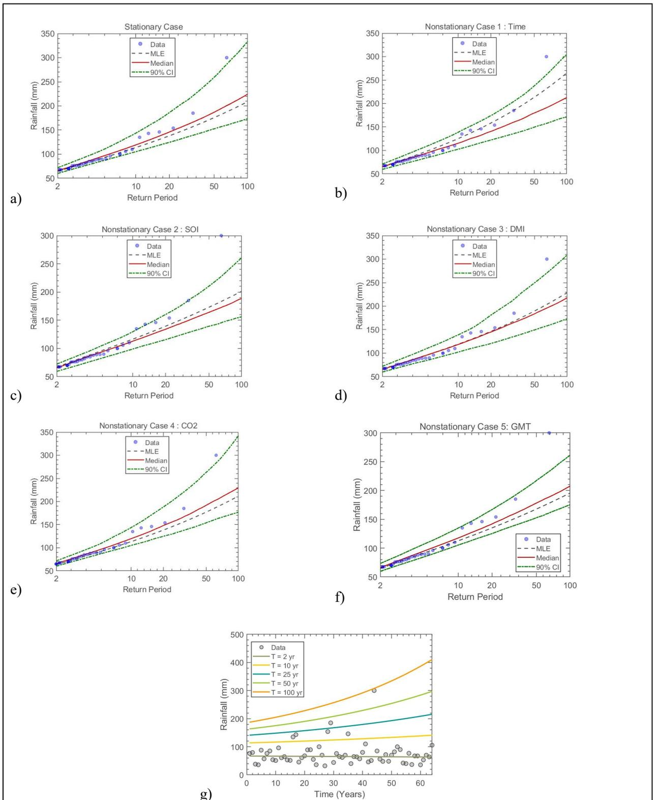
Figure 7.39 The GEV (a) stationary model, (b) non-stationary model considering time as a covariate, (c) non-stationary model considering SOI as a covariate, (d) non-stationary model considering DMI as a covariate, (e) non-stationary model considering CO<sub>2</sub> as a covariate, (f) non-stationary model considering GMT as a covariate and (g) effective return period as a function of time for Station 154: Mkuze – Mkuze Estate
