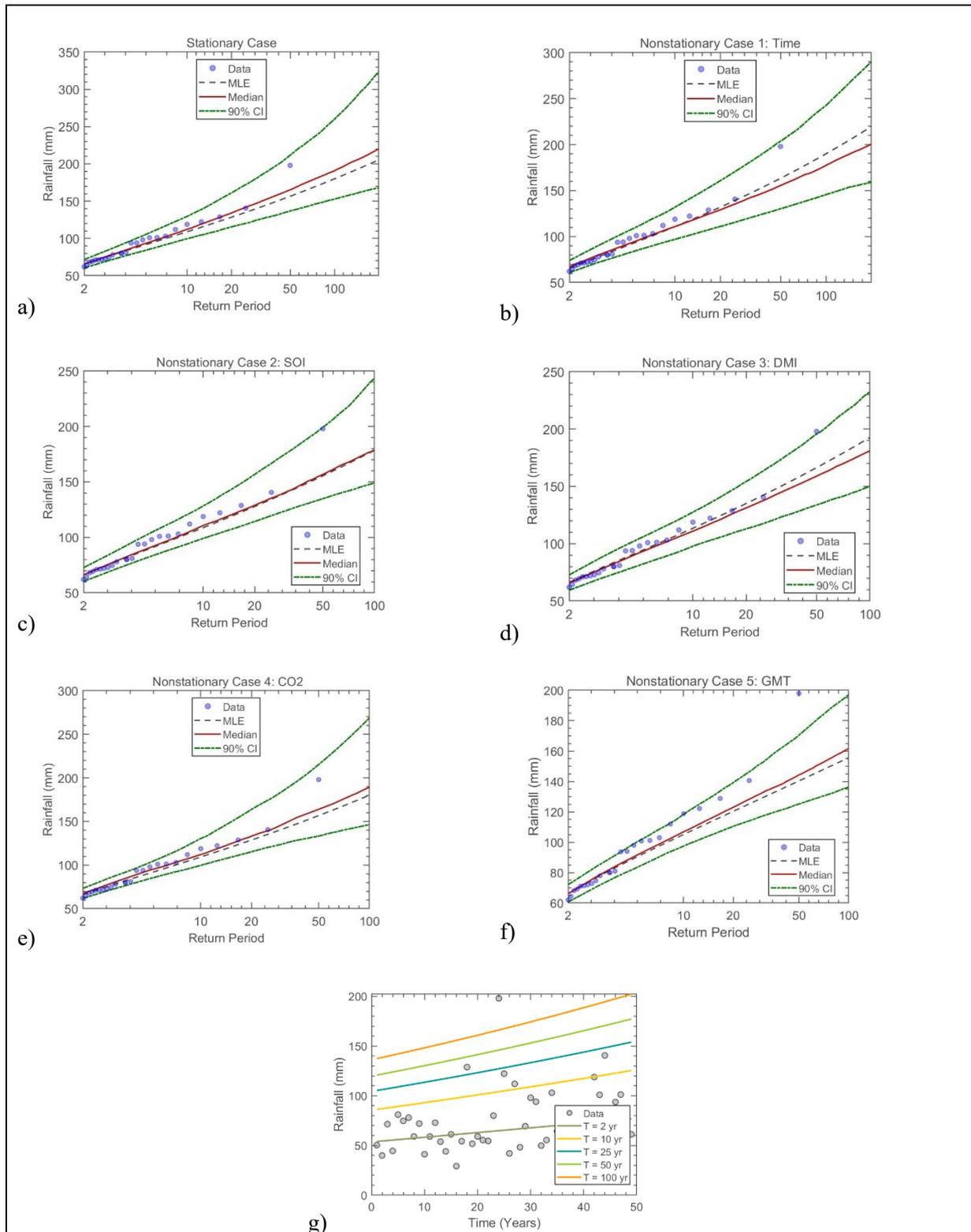
Figure 7.2 The GEV (a) stationary model, (b) non-stationary model considering time as a covariate, (c) non-stationary model considering SOI as a covariate, (d) non-stationary model considering DMI as a covariate, (e) non-stationary model considering CO<sub>2</sub> as a covariate, (f) non-stationary model considering GMT as a covariate and (g) effective return period as a function of time for Station 6: Pongola – SASRI
