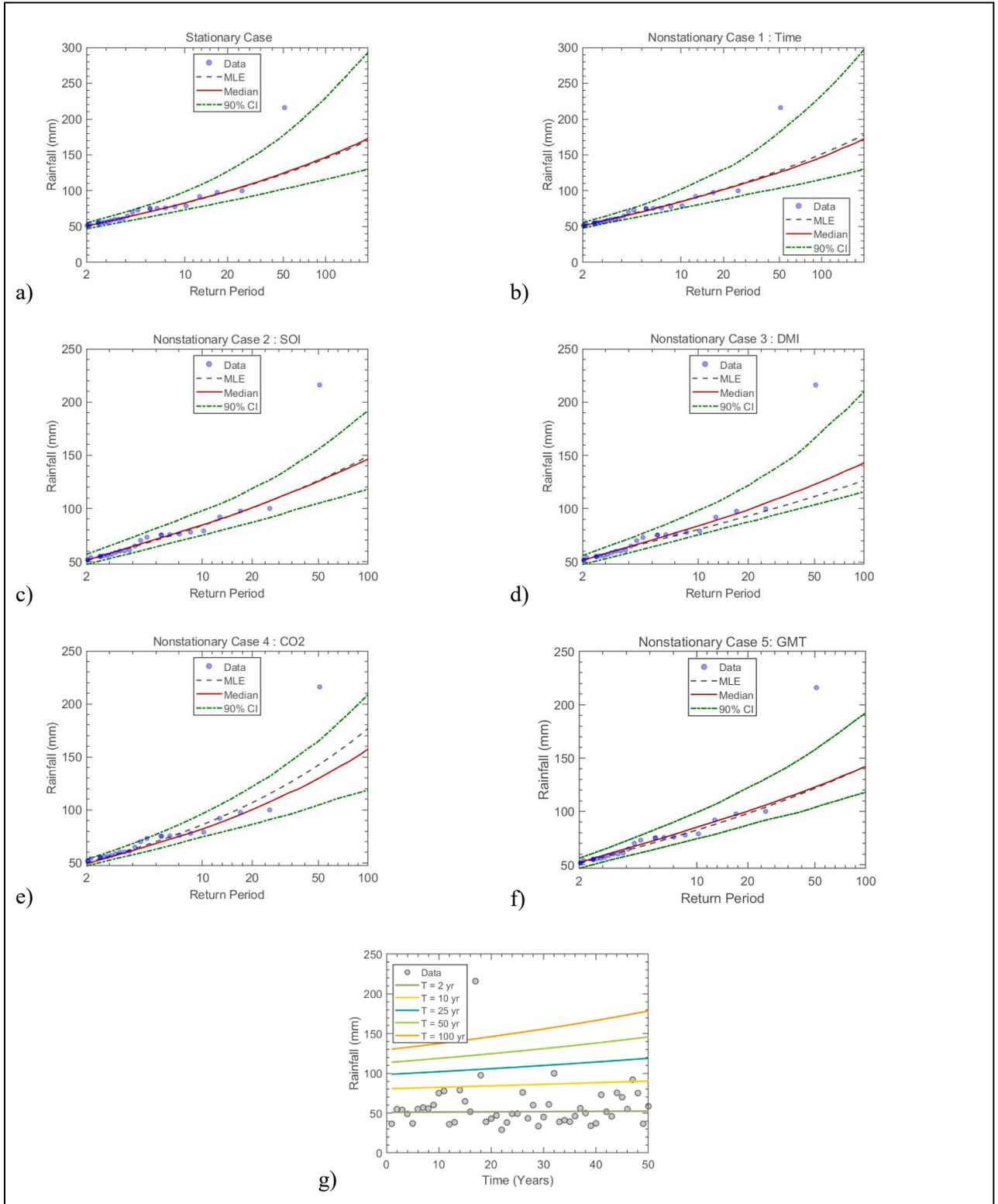
Figure 7.10 The GEV (a) stationary model, (b) non-stationary model considering time as a covariate, (c) non-stationary model considering SOI as a covariate, (d) non-stationary model considering DMI as a covariate, (e) non-stationary model considering CO<sub>2</sub> as a covariate, (f) non-stationary model considering GMT as a covariate and (g) effective return period as a function of time for Station 23: Noodsberg – Illovo Sugar Mill
