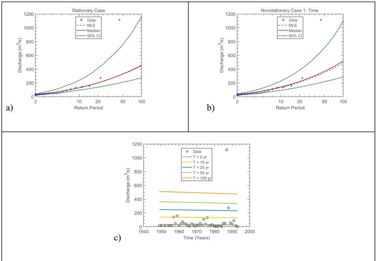
Figure 8.3 LP3 (a) stationary model, (b) non-stationary model considering time as a covariate, and (c) effective return period as a function of time for Station: U2H001
