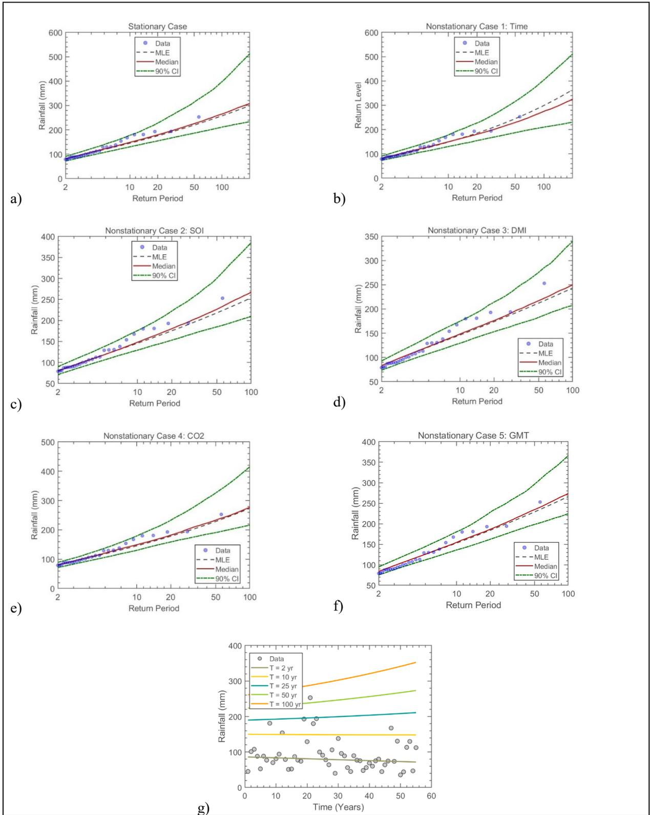
Figure 7.3 The GEV (a) stationary model, (b) non-stationary model considering time as a covariate, (c) non-stationary model considering SOI as a covariate, (d) non-stationary model considering DMI as a covariate, (e) non-stationary model considering CO<sub>2</sub> as a covariate, (f) non-stationary model considering GMT as a covariate and (g) effective return period as a function of time for Station 8: Glen Park – St Lucia Farms
