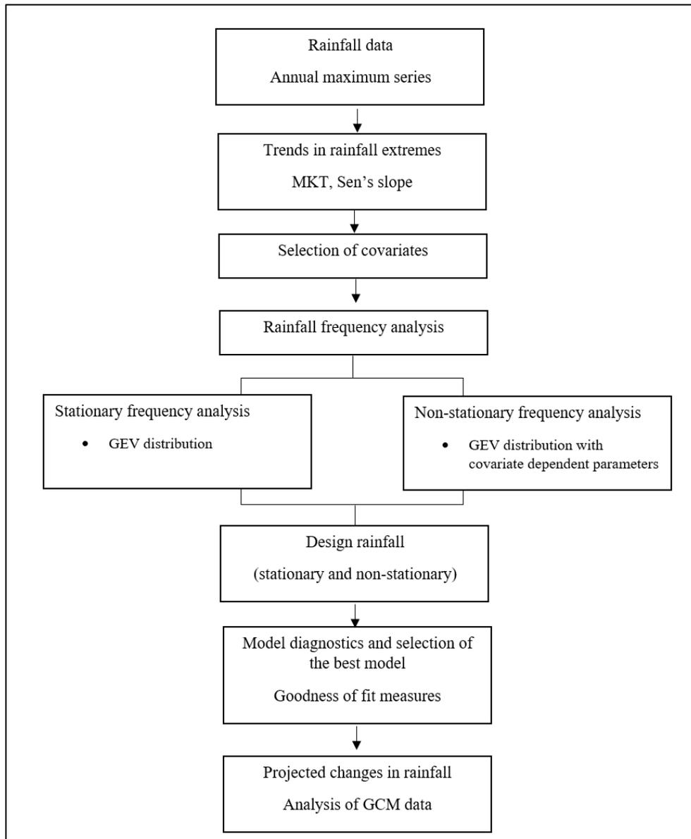
Figure 2.2 Stationary and non-stationary design rainfall estimation procedures
