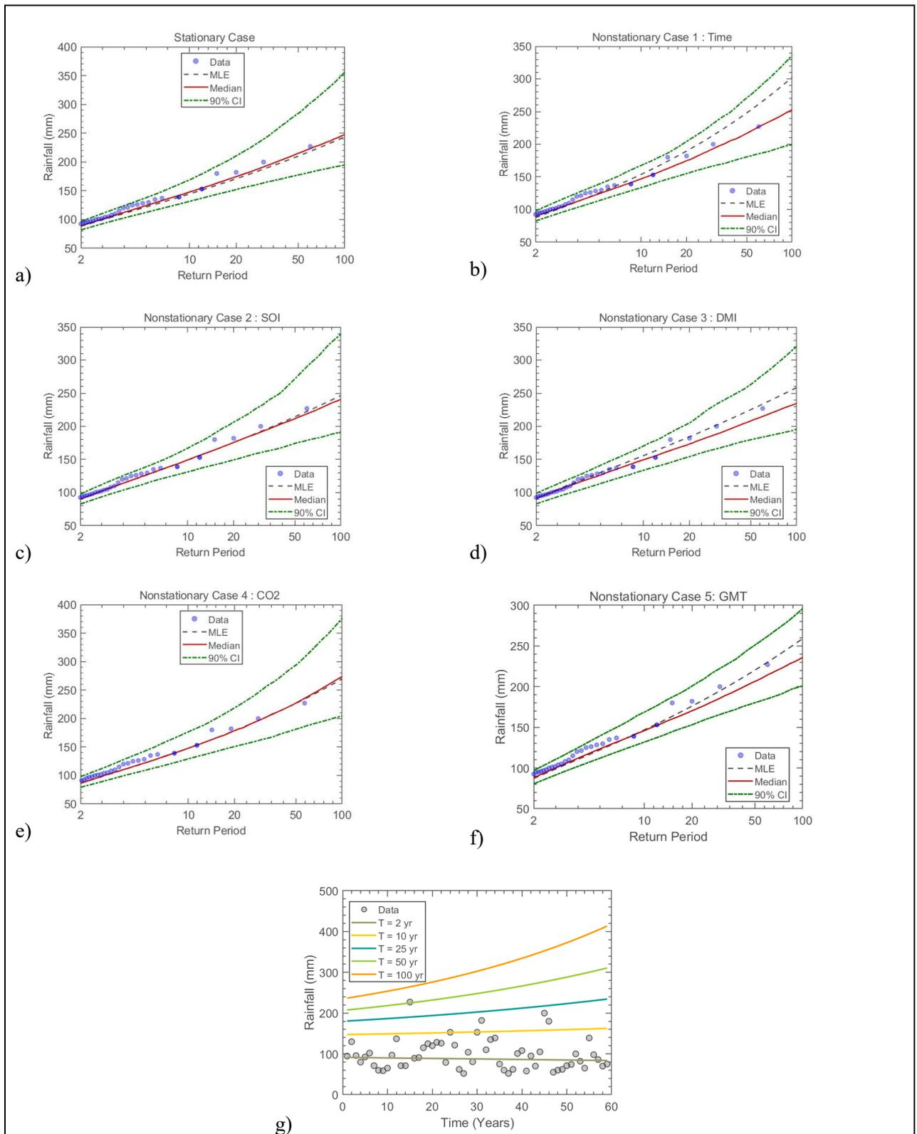
Figure 7.26 The GEV (a) stationary model, (b) non-stationary model considering time as a covariate, (c) non-stationary model considering SOI as a covariate, (d) non-stationary model considering DMI as a covariate, (e) non-stationary model considering CO<sub>2</sub> as a covariate, (f) non-stationary model considering GMT as a covariate and (g) effective return period as a function of time for Station 132: Tugela Mouth – Wetherly Estate
