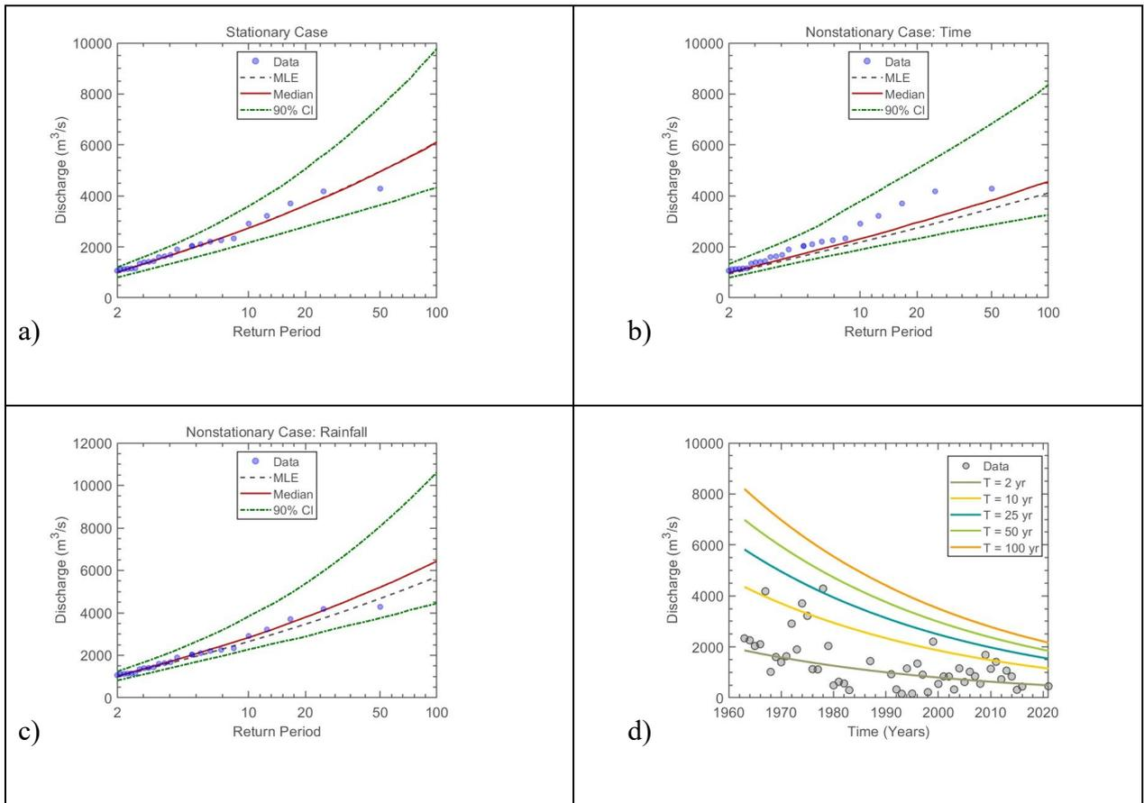
Figure 8.10 LP3 (a) stationary model, (b) non-stationary model considering time as a covariate, (c) non-stationary model considering rainfall as a covariate, and (d) effective return period as a function of time for Station:V5H002
